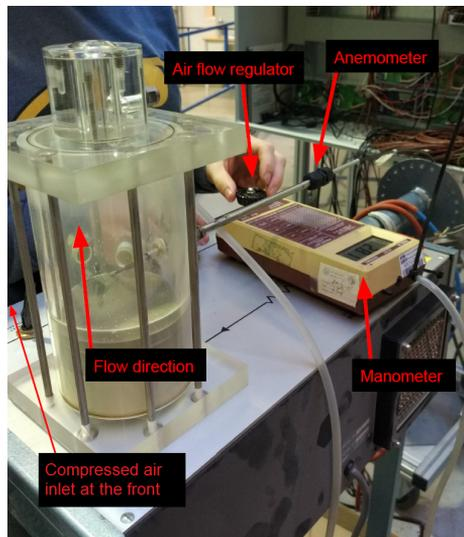
*Figure 3.8: Calibration setup for anemometer calibration*
