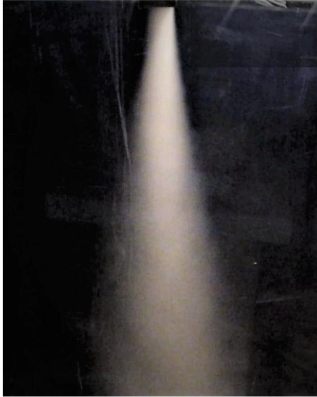
*Figure 3.2: Smoke visualization of the jet's profile*
