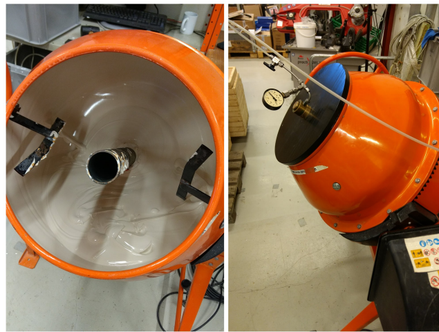
Figure F.1: Slurry after mixing is completed (left) and concrete mixer (right)
