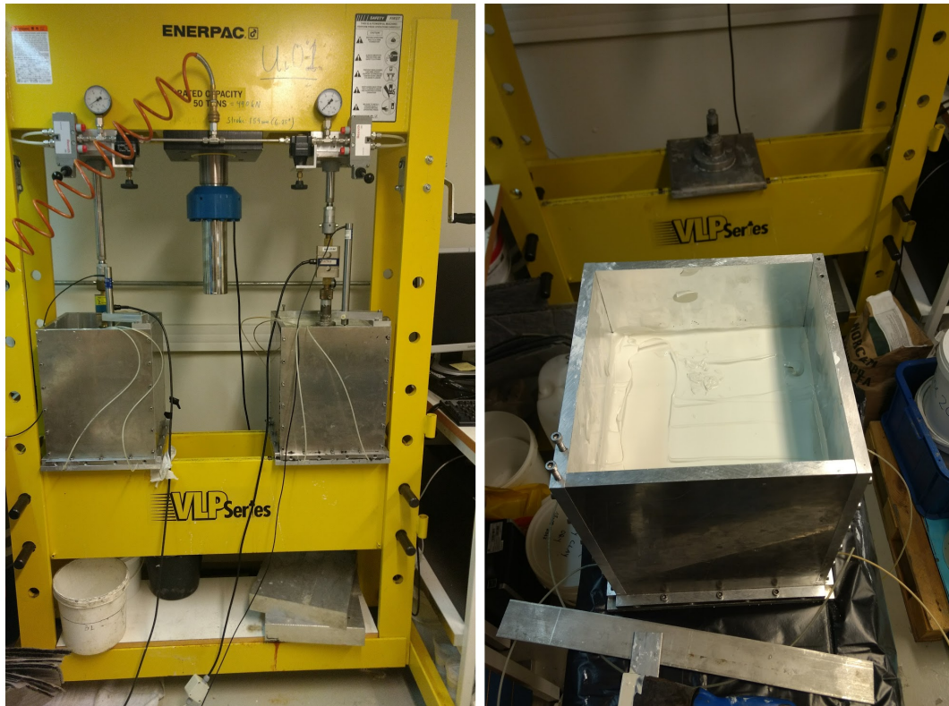
Figure F2: Consolidation boxes installed (left) and slurry placed in consolidation box (right)
