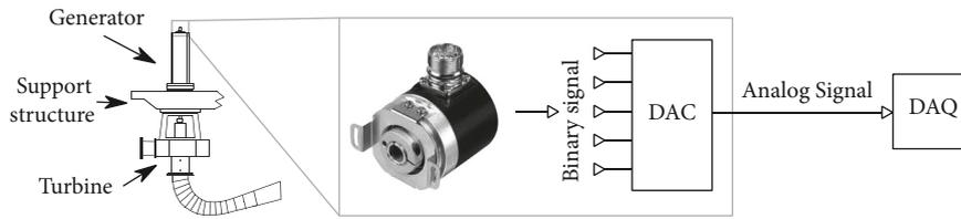
FIGURE 3: Absolute position sensor on the shaft end above the generator.
