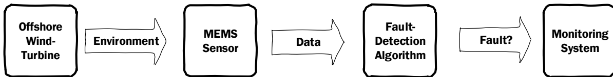
Figure 2.1: The WiVind project at a highly conceptual level. A sensor gathers data about the surrounding environment and feeds the data into an algorithm. The algorithm allows a monitoring system to know whether the blade is faulty or not.
