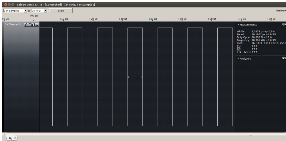
Figure 8.1: Toggling a pin through the virtual Linux file system sysfs.
