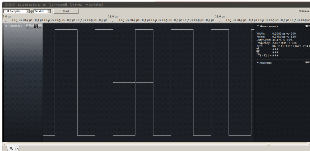
Figure 8.2: Toggling a pin through memory mapping.
