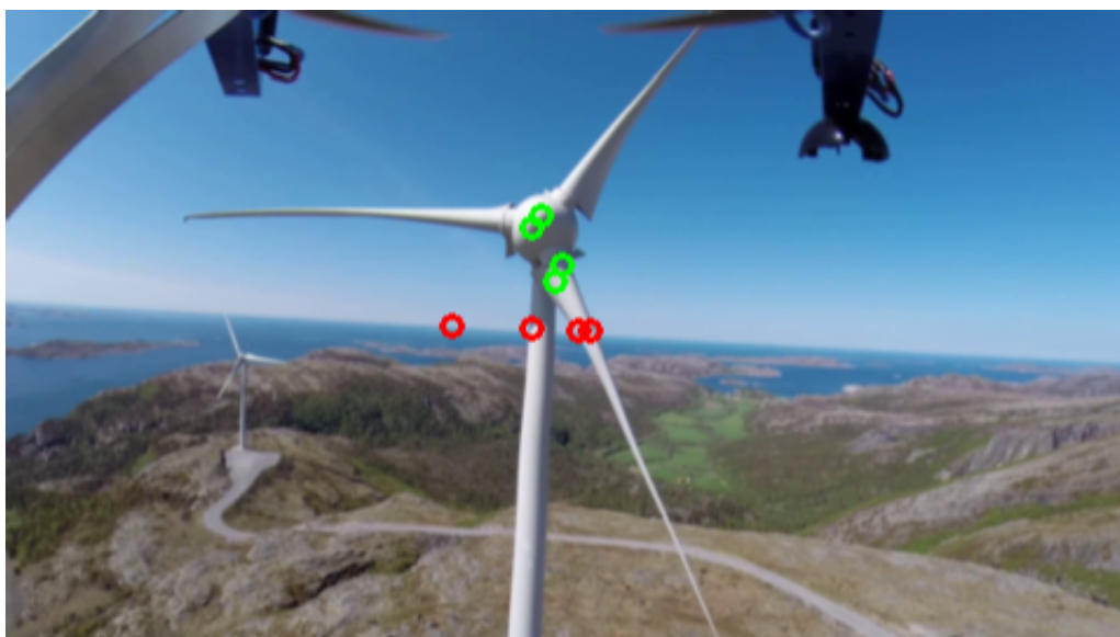
Figure 6.9: In this case there were some bad intersection points due to the horizon being detected as a blade line. The red circles show intersection points which were removed by posed restrictions, leaving the better green points for the calculation of average.
