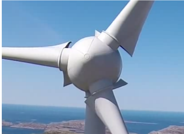
Figure 7.4: An example on what the starting position might look like when the blade inspection program is initiated.
