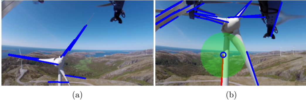
Figure 9.2: (a): Failed detection because the tower does not exhibit any lines which are long enough to be detected. (b): Failed detection because the highest point among the tower lines (blue circle) is not high enough and thus the blade search radius (green) does not capture any of the blades.
