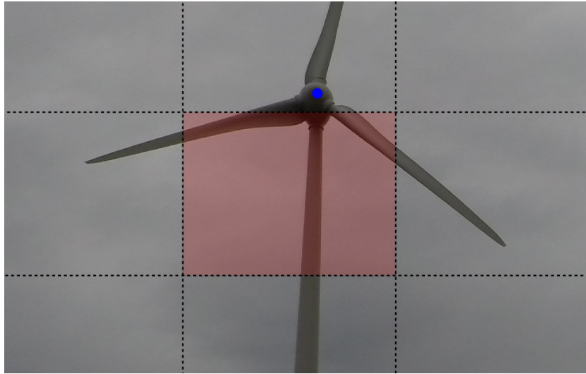
Figure 7.2: The red rectangle illustrates the boundary in which the UAV attempts to keep the target (blue dot). In this example it is clear that the target is above the upper bound, and the UAV will fly upwards as commanded by T1.
