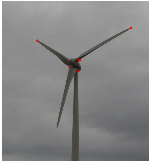
Figure 6.2: The red circles show the detected corners using the Harris corner detector on the image from figure 6.1a.
