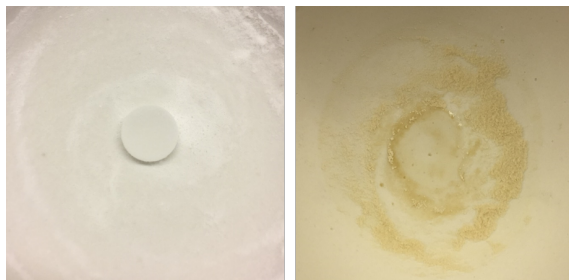
Figure 4.4: Pictures showing a successful (left) and a failed (right) hydrophobicity test.
