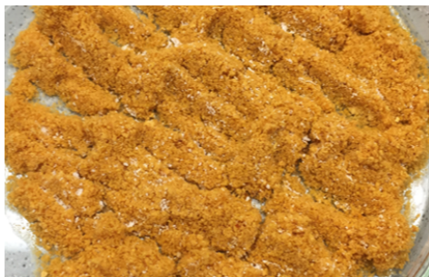
Figure 4.8: Small crystals were observed in CP-0.1(III)-Sulf .
