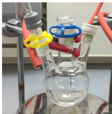
Figure 3.3: Experimental setup used for inert atmosphere.
