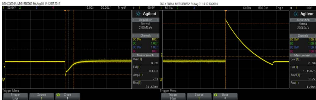
Voltage drop and overshoot with 4A test current
