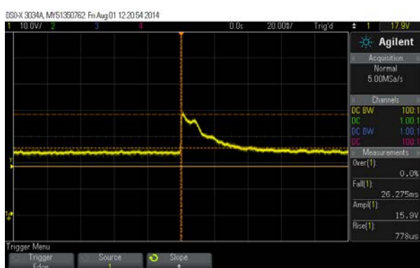
Voltage overshoot with 1A test current
