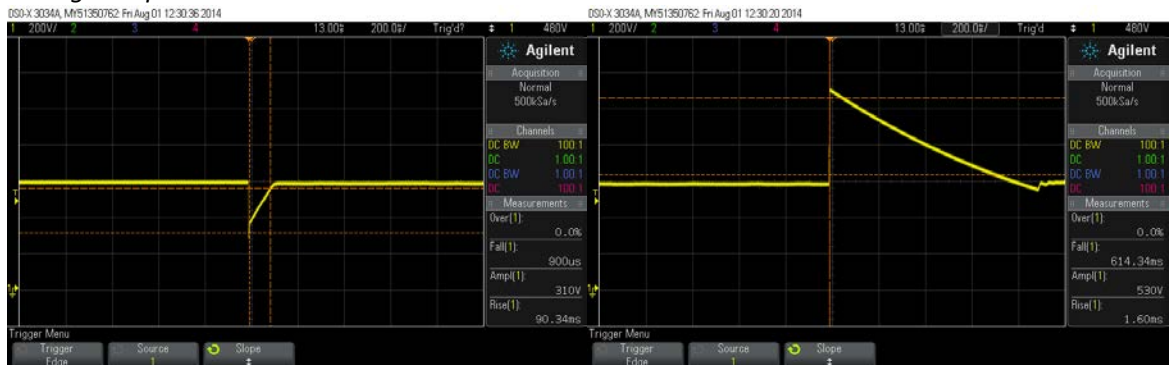
Voltage drop and overshoot with 6.5A test current
