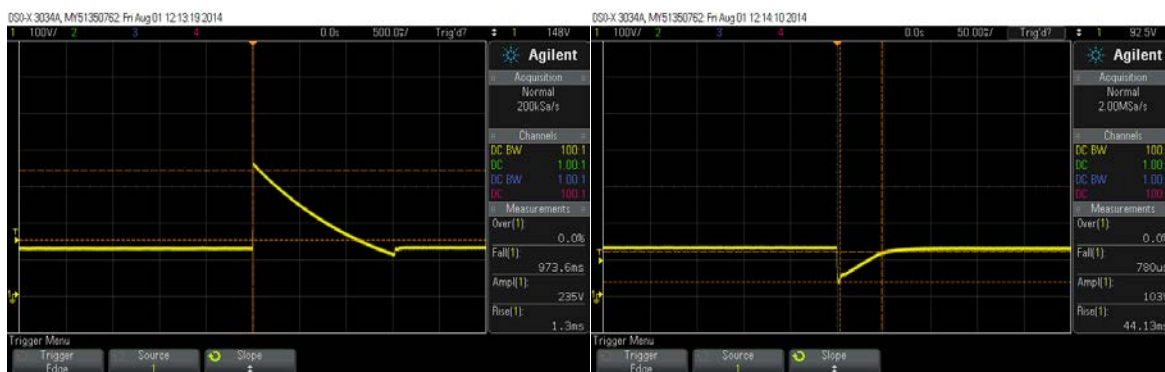
Voltage drop and overshoot with 3A test current
