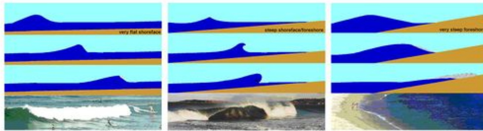
Figure 2.12: Depth-induced wave-breaking: spilling, plunging and surging [14]
