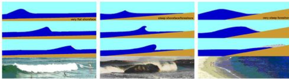
Figure 1.5: Depth-induced wave-breaking: spilling, plunging and surging [7]
