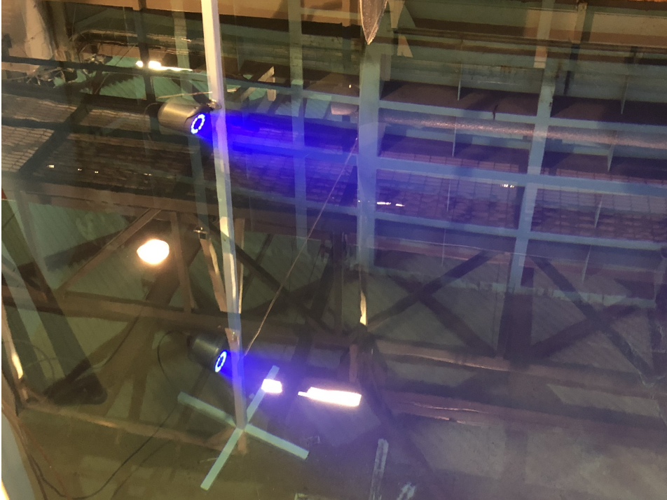
Figure 4.3: Two of the four Ocus Underwater Cameras used to track the descending structure.
