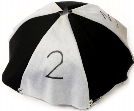
(a) Parachute A3 from [10]. The parachute has a diameter of 0.79 of structure length and is not optimized for the dropped structure. Image from [10]
