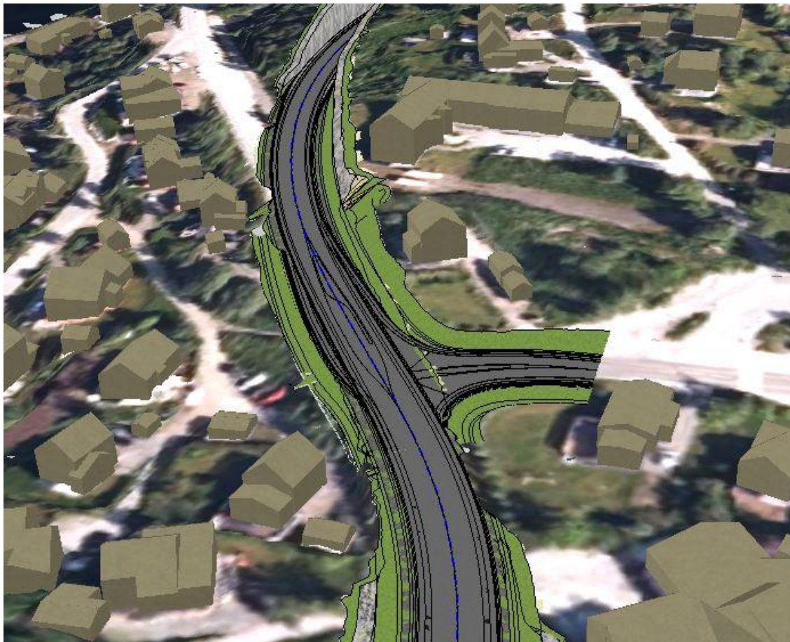
Figur 35: Kryssutforming E6/fv.830 i Novapoint
