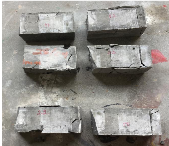
Figure 7-5: After compressive strength test for 1% fibre content
