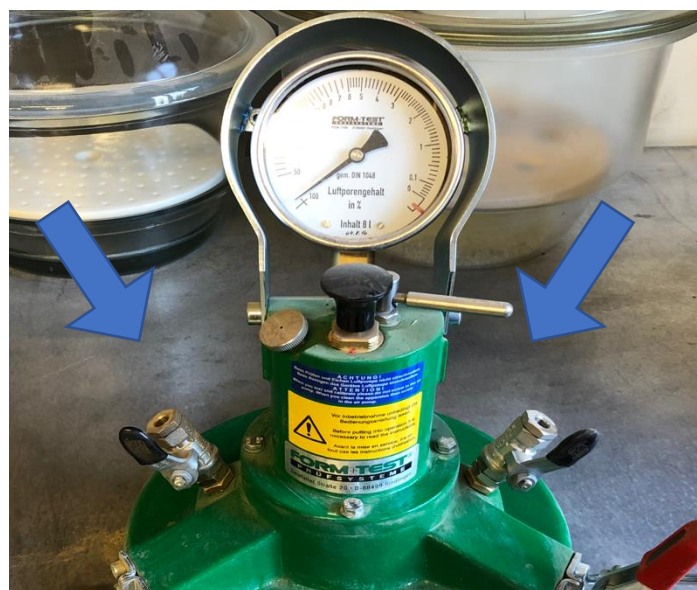
Valve A and Valve B
