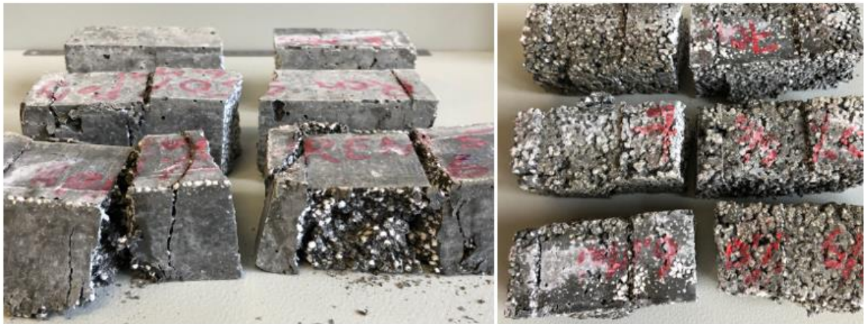
Figure 7-10: 50% polystyrene after the compressive strength tests
