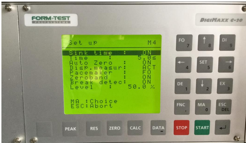
Figure 6-9: Digital screen for reading the measurements of flexural and compressive strengths
