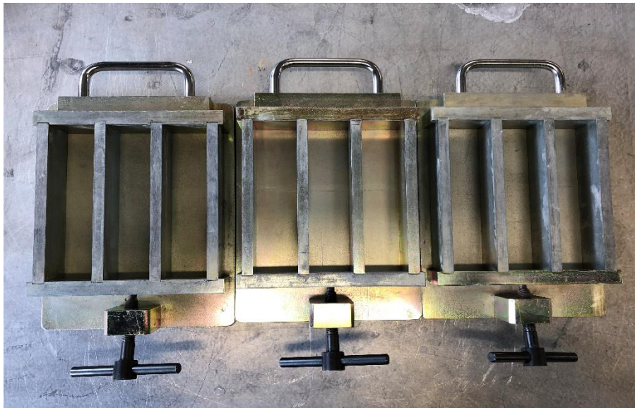
Figure 6-4: Prisms ready for cement paste to be poured in
