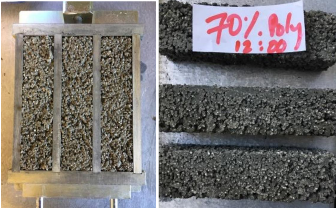
Figure 7-9: 70% Polystyrene, removed from the casting mould after 24 hours, ready to be put in the water bath
