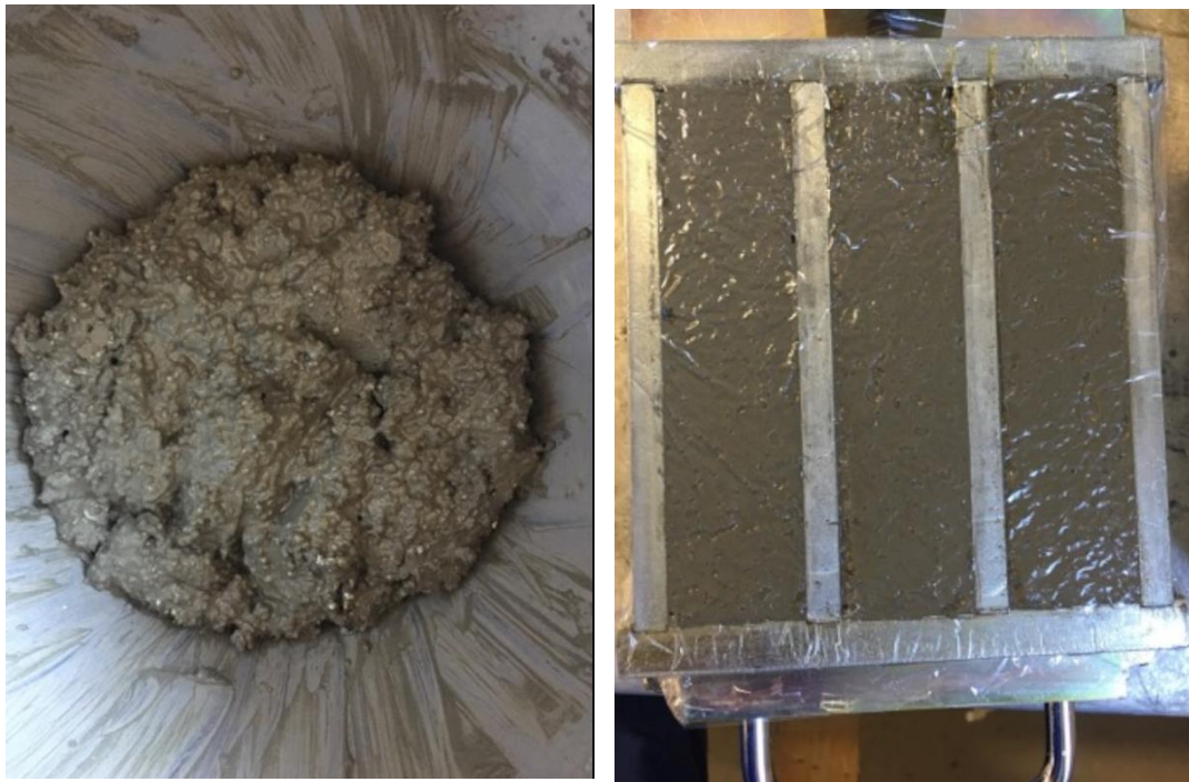
Figure 7-8: Image on the left shows the mixture of 50% polystyrene, while image on the right shows the same mixture but, in the mould, ready to harden at room temperature
