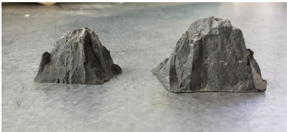
Figure 7-3: After compressive strength test for reference samples, shows that it is a good mix, very small air bubbles are observable
