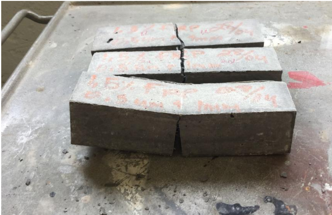
Figure 6-11: Halved rectangular shaped samples ready for compressive strength tests
