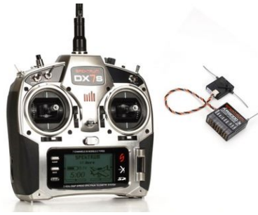
Figure 2.2: The 7-channels RC transmitter Spectrum DX7s with receiver. Retrieved from http://hobbyfly.com .
