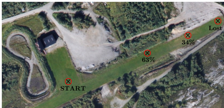
Figure 2.4: The range of the original wifi module at the PandaBoard was tested in field. The airstrip at the picture is approximately 200 meters from start to the end of the runway where the communication was lost. The map data is retrieved from http://norgebilder.no
