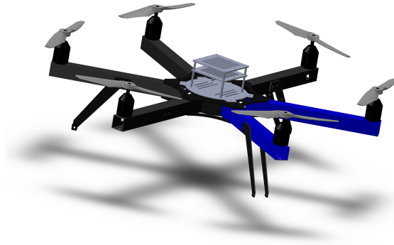
Figure 1.1: The 3DR ArduCopter Hexa is a multicopter designed and manufactured at the 3D Robotics headquarters in San Diego, California. The model is rendered by Kristian Klausen.
