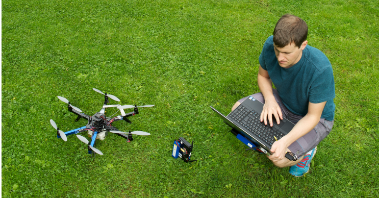
Figure 8.3: The operator monitors the multicopter’s status, mission and watches the video stream for objects, responsible for sending a manual detection.
