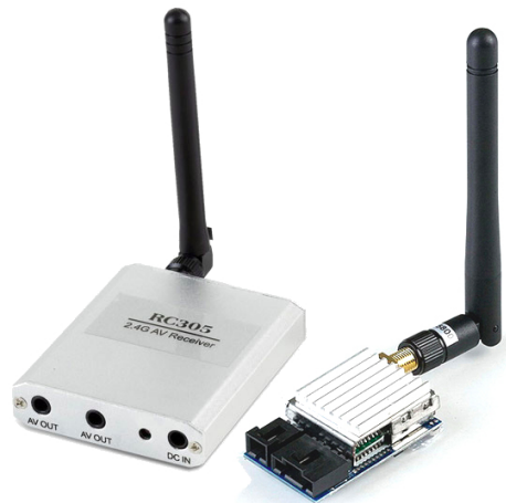
Figure 2.7: 5.8 GHz 200 mW FPV wireless AV Tx and Rx set. It has a range at 500 m with the supplied antenna. An optional directional antenna can extend the range to over 1 km. Retrieved from http://www.uavobjects.com
