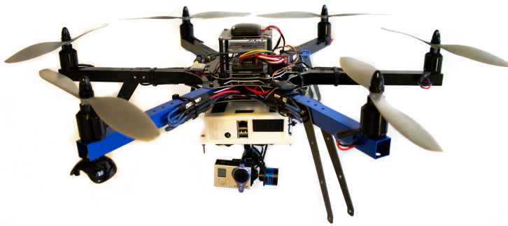
Figure 2.1: The hexacopter 3DR ArduCopter Hexa mounted with the SAR payload. The white box contains the computational unit and act as a platform for the gimbal. The payload and gimbal are discussed later in the section.
