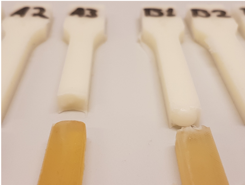
Figure 20: The interfacial curvature change of the adhesion testing between samples A and B.
