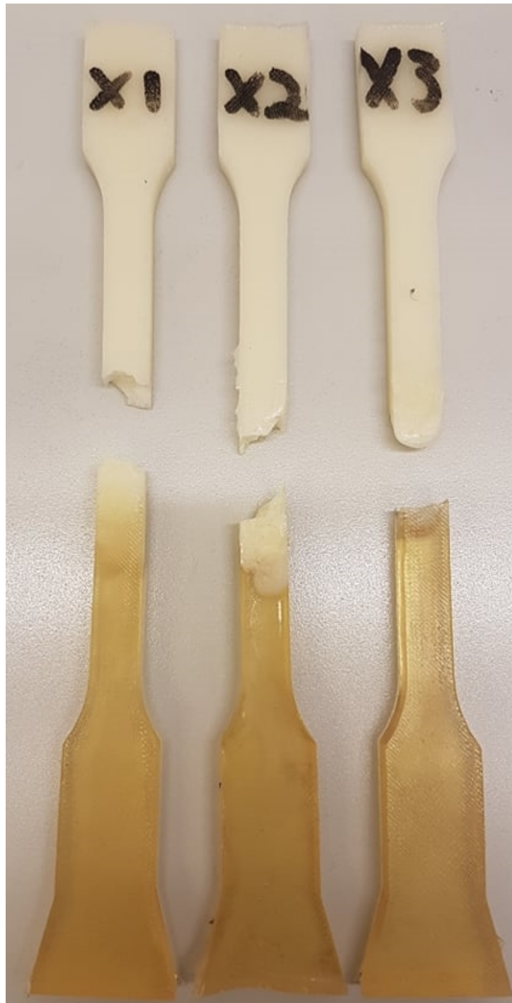
Figure 12: Mixed interface adhesion testing samples after results were gathered.
