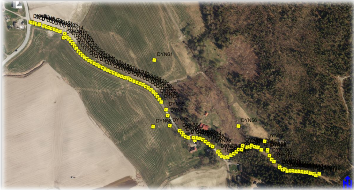
Figure 37 - Orthophoto with dynamic RTK-measurements
