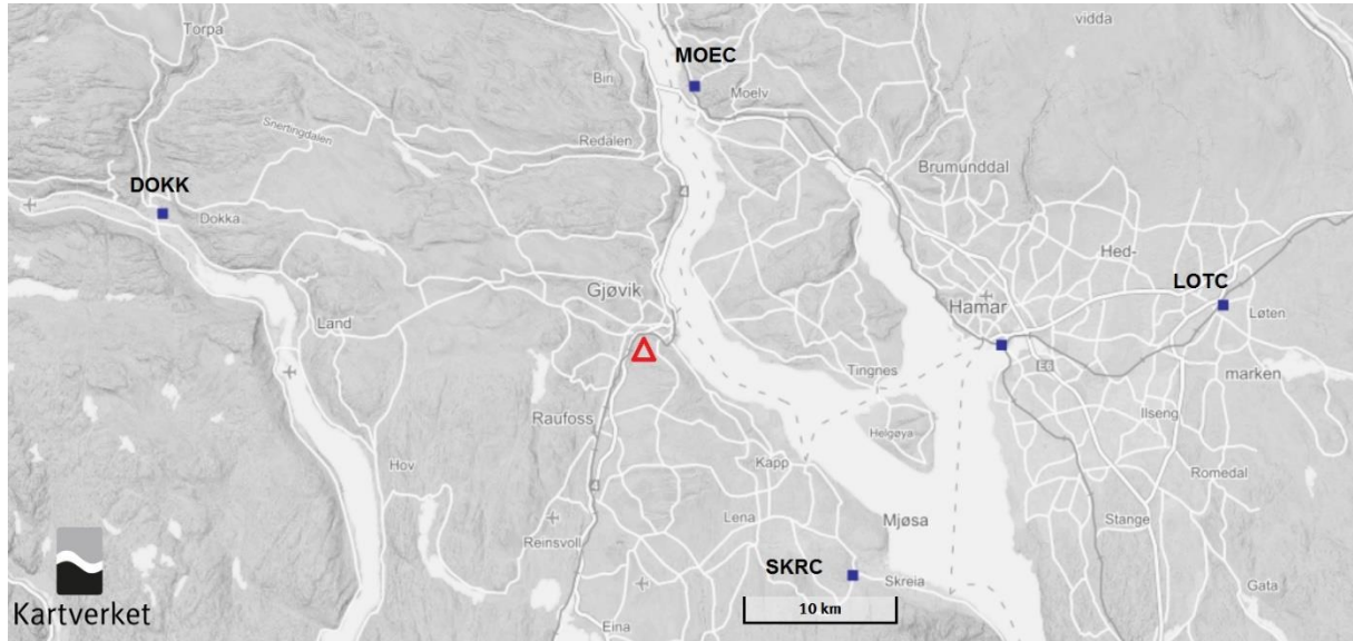
Figure 28 - map with overview of the base stations we used in our networks and the approximate location of our benchmarks marked with the red triangle
