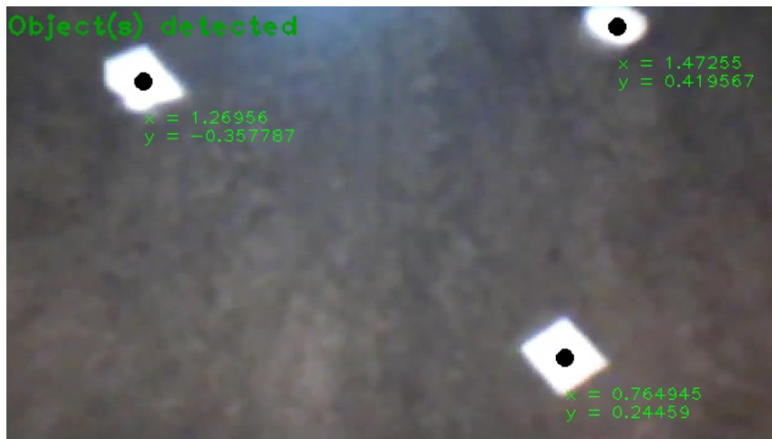
FIGURE 7.6: Test of back-projection using fixed orientation and camera position.
