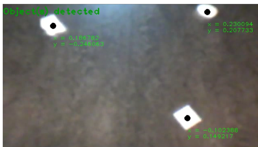
FIGURE 7.7: Test of simplified method using fixed orientation and camera position.
