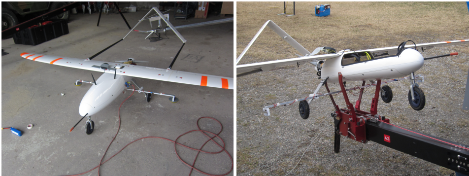
(c) Overview of the bar mounted on the Penguin B. (d) The Penguin B, with the bar, placed on the launch catapult.
