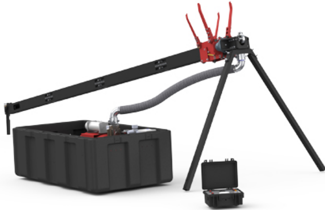
Figure 2.5.: Portable Pneumatic Catapult, used to launch the Penguin B. [12]
