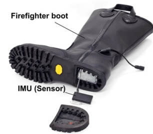
Figure A.2: IMU embedded in the heel of a firefighter boot. Courtesy of [51]
