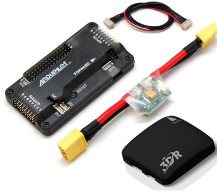
Figure 3.2: APM 2.6 with a voltage regulator and an external magnetometer and GPS module Courtesy diydrones.com
