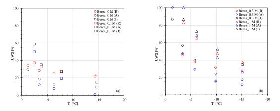
Figure 4. UWS estimates of EMT-SCA joint methods (Berea: Berea sandstone; 0~1 M: Salinity; R: Resistivity results; A: Acoustic results; J: Joint method results)
