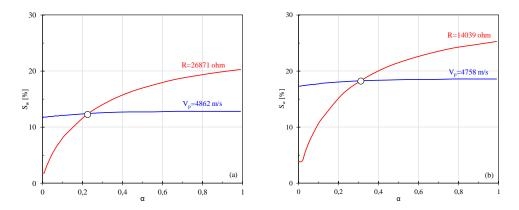
Figure 3. Numerical solution of ( $\alpha$ ,  $S_w$ ) according to R = 26871  $\Omega$ m,  $V_p$  = 4862 m/s (a) and R = 14039  $\Omega$ m,  $V_p$  = 4758 m/s (b)
