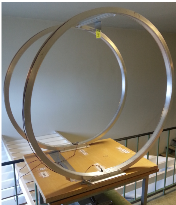
Figure 4.11: The Helmholtz Coil made in [3]. Can be used to test the ADCS Prototype
