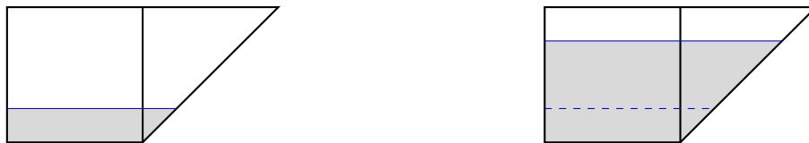
Figure 3.6: The change of signed area in square and triangular hysteron cells with an increasing input. While the change in the square cells is linear, the signed area of the triangular cells increases more rapidly.
