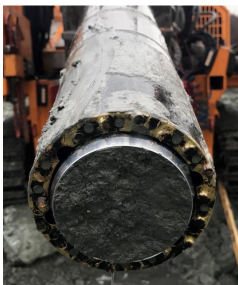
Figure 35. Example of GP-Tr sample of stabilised Klett clay.
