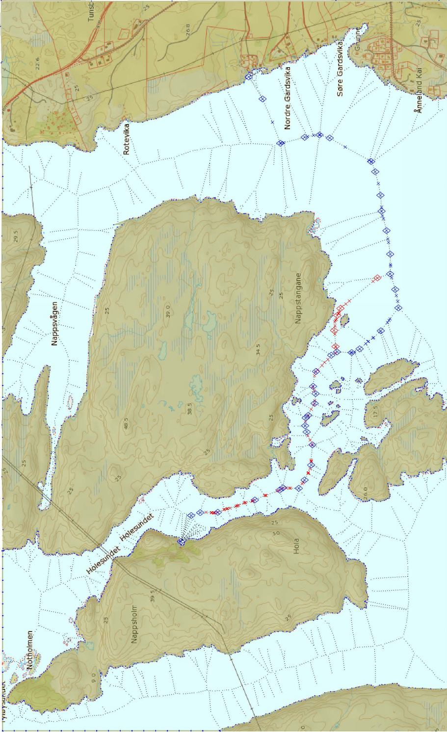
Figure 6.7: Step5: The second shortest path is now undergoing the same procedure. The number of waypoints is reduced and clearance check is performed.
