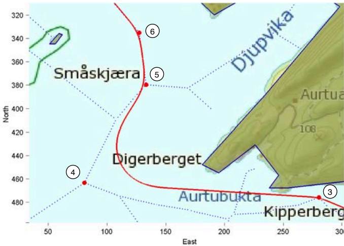
Figure 6.12: A depiction of how the final path is based on the selected waypoints, while at the same time it does not cross all of them. However, the clearance constraints are always satisfied although the path is an approximating one.
