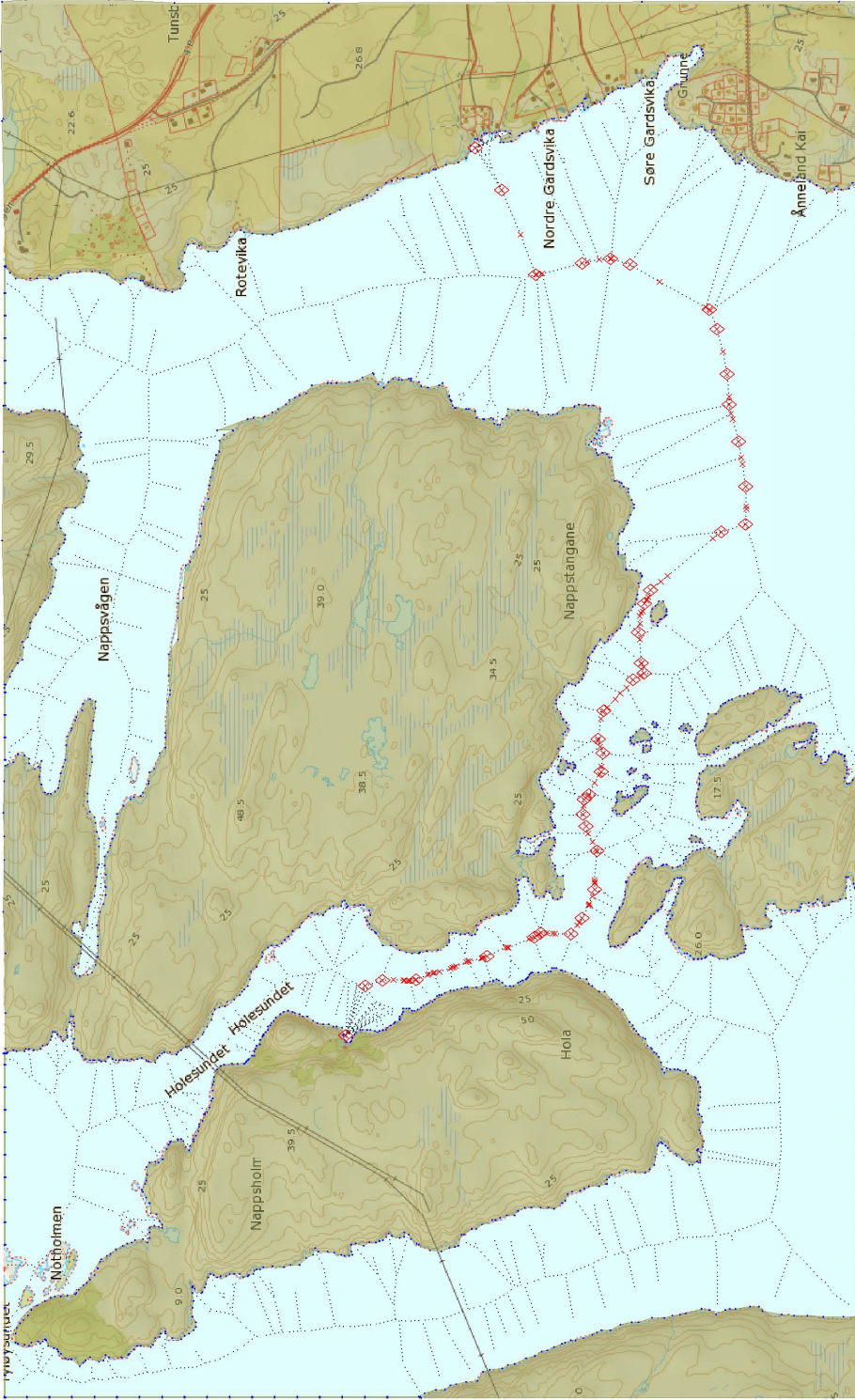
Figure 6.5: In Step 3, the inline, or almost collinear waypoints are removed (only the diamond-shaped points are kept) and a clearance check is performed.
