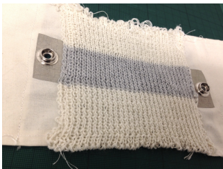
Figure 4: Stretch sensor, knitted from stainless steel and polyester yarn.
