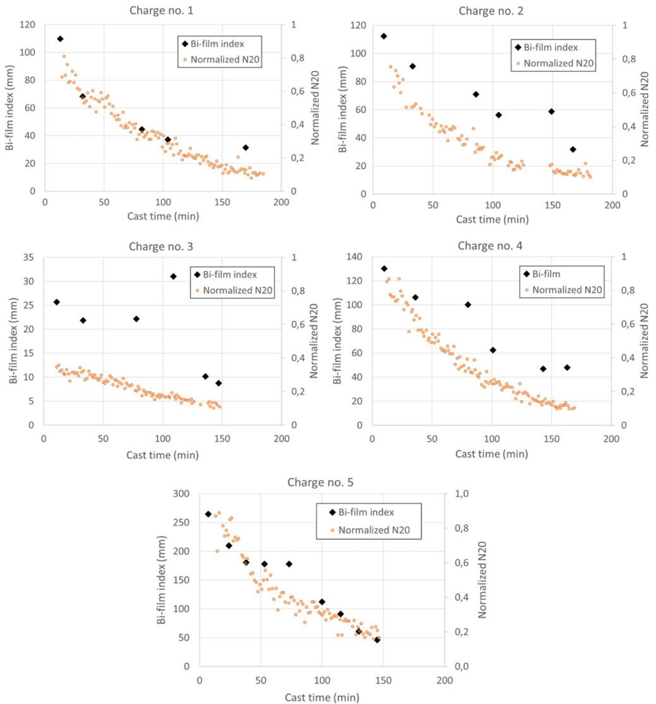
**Fig. 6** The bi-film index and LiMCA versus casting time is plotted for 5 charges
