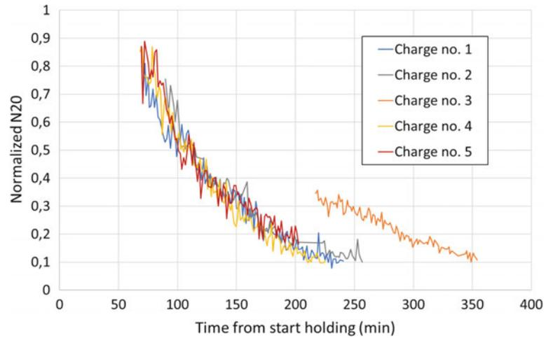
**Fig. 8** Bi-film index plotted from start of the holding for the 5 charges, showing variation in bi-film index values
