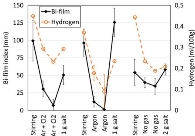
**Fig. 3** Influence of various melt treatments on hydrogen and bi-film index. Each measurement series correspond to one of the three crucibles in the parallel setup. The three first hydrogen measurements in the second series (with error bars) are the average value of two analysis. The end points of these error bars give the value of these two analysis
