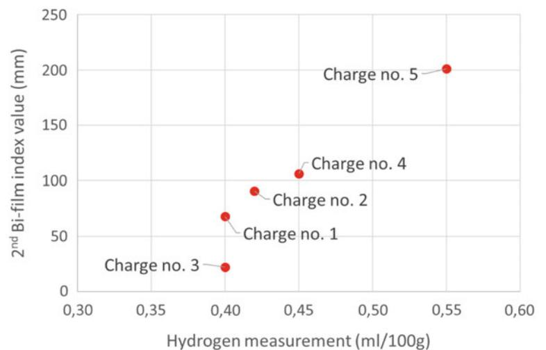
also shows a positive correlation between hydrogen and the bi-film index. This indicates that a bi-film index measurement can be used as a melt quality indicator; a low bi-film index means high quality and high bi-film index means bad quality. Additional measurements are then needed to determine the reason for the bad quality.
