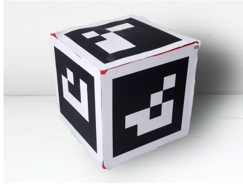
Figure 4.22: Aruco Merger: Photo of marker cube
