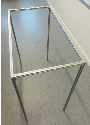
Figure 4.7: Photo of test rig: The rig's measurement is 1x1x0.5 meters.
