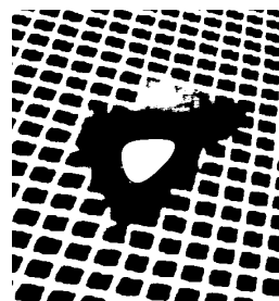
Figure 4.20: Picture showing adaptive threshold performed on the picture from fig. 4.17, using mask size: 175x175
