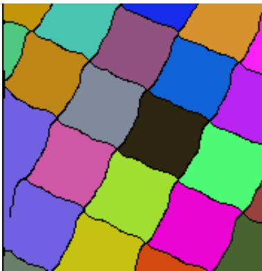
Figure 4.7: Picture showing the test image after it is run through the large mask analysis using Bilateral blur - 3x3 mask
