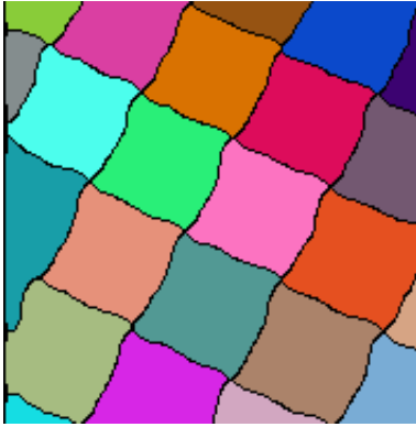
Figure 4.4: Picture showing the test image after it is run through the large mask analysis using Gaussian blur - 3x3 mask
