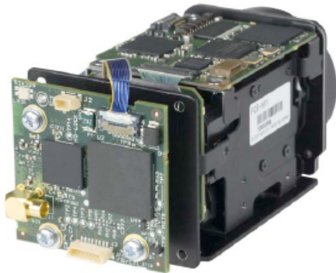
Figure 3.2: Intertest EM15710 iShoot-FCB-HDSDI interface, from Intertest [13].
