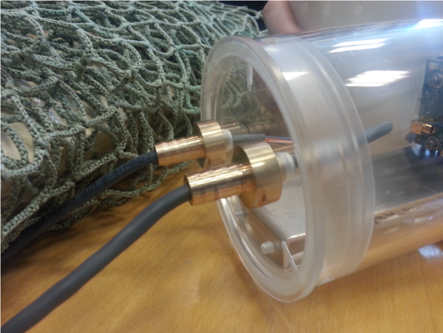
Figure 6.3: Same housing as shown in figure 6.2 but showing the nipples for the waterproof cable entries.
