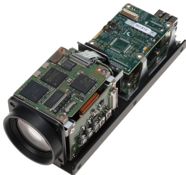
Figure 3.4: Pleora SB-Pro IP Engine for Sony FCB-H11, from Intertest [14].
