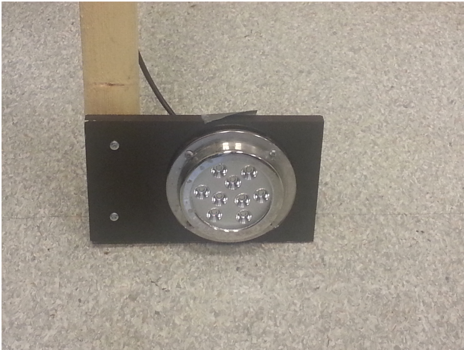
Figure 6.4: Underwater LED lights mounted on a plywood backing plate.
