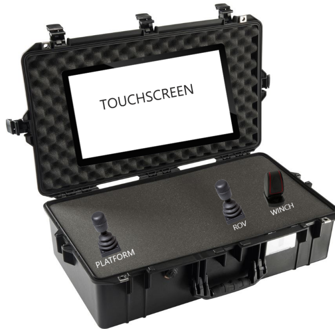
Figure 3.4: Dedicated control station
