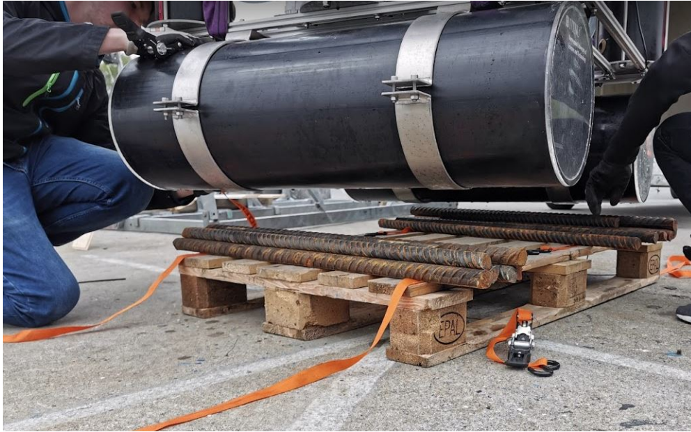
Figure 4.25: Lowering center of gravity
