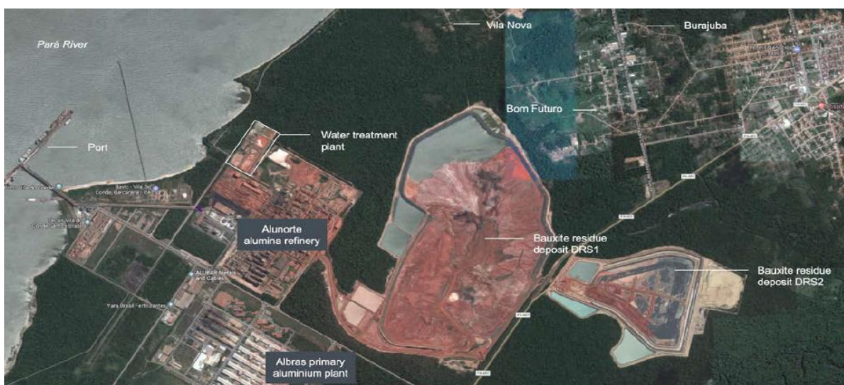
Figure 5: Barcarena site layout Source: Hydro (2019b, p. 72)
