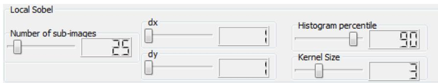
Figure 31: Local Sobel segmentation parameters, System 1
