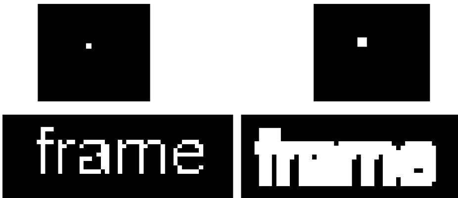
Figure 12: Morphological dilation. Before(left column) and after(right column)
