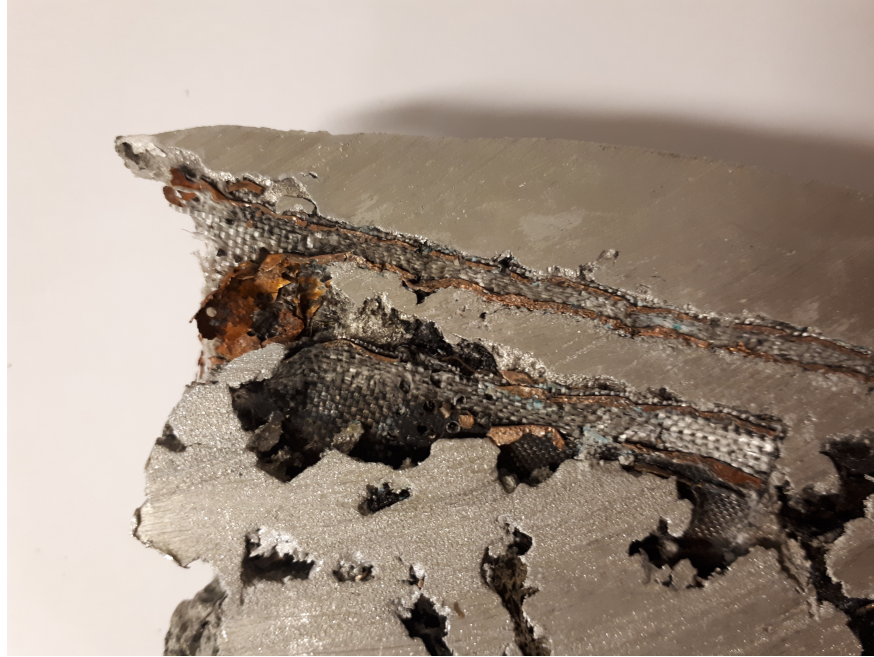
Figure 47: Cross section of a solidified sample with a PCB trapped in the Al. There is visible Cu between the fiberglass layers that has not dissolved because of the glass fibers.
