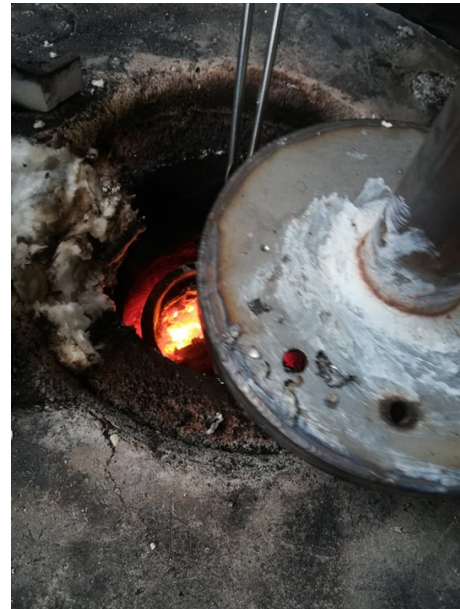
Fig. 2. Photo of an experiment with smartphones in liquid aluminium
