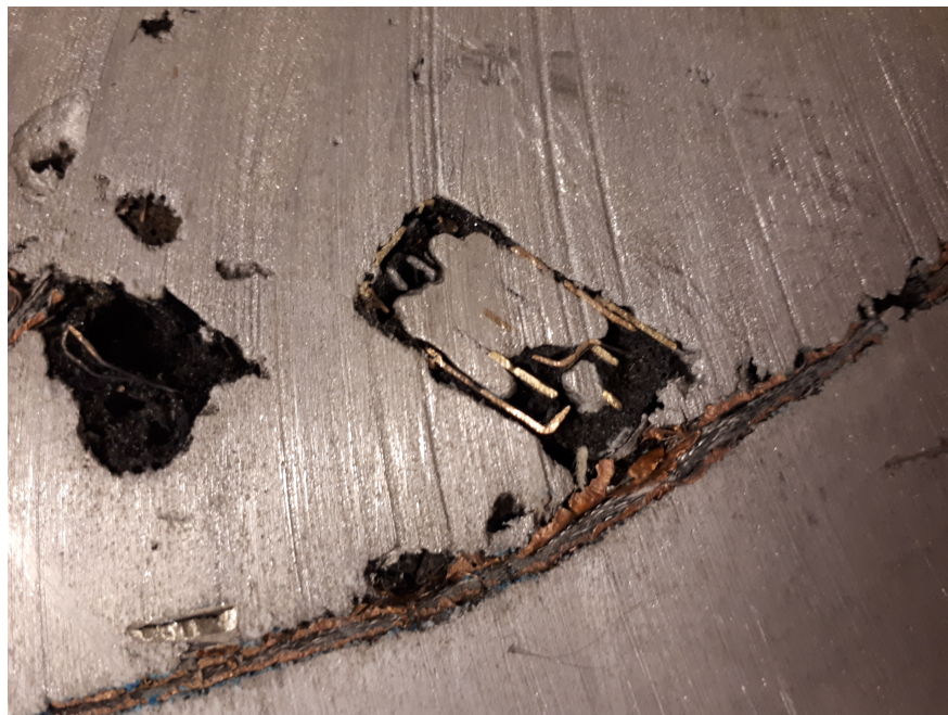
Figure 48: Cross section of a solid sample containing a EC still connected to the PCB. There are traces of organic residue inside the EC.
