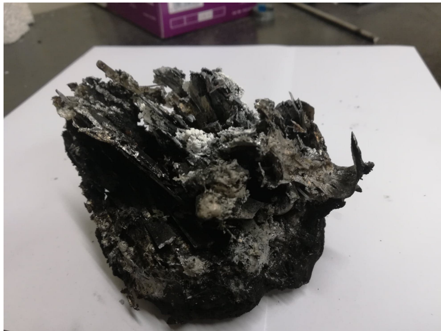
Figure 49: The zirconia ceramic filter with remains of the smartphone and Al.
