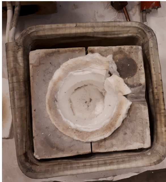
Figure 14: The electromagnetic coil seen from above. The inside of the coil is isolated for preventing the Al to solidify too fast.
