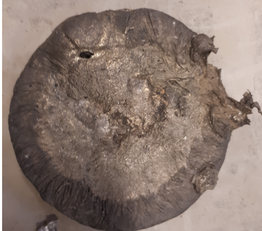
Figure 34: Picture of the remaining melt, after cooling inside the electromagnetic field of the coil. The picture is taken from above. The dross has a different colour closer to the edge than towards the center.
