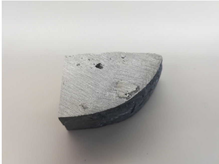
Figure 29: A piece of metallic Nd not completely dissolved during the trial, close to the bottom of the sample.
