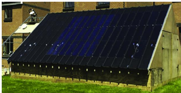
Figure 28: Heat mat experimented as a building integrated material during DECC's investigation in Cardiff [2].
