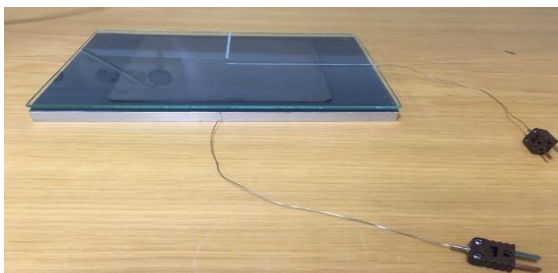
Figure 3: PV/T system with PVC pad as TIM. This unique system-design was void of rear glass in the PV system.
