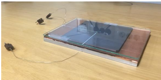
Figure 2: PV/T setup with copper tape as TIM.
