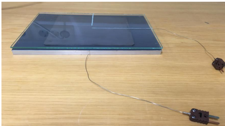
Figure 38: Specimen setup for scenario B. The PVC pad can be seen through the transparent glass layer. Two thermocouples can also be seen in the figure.
