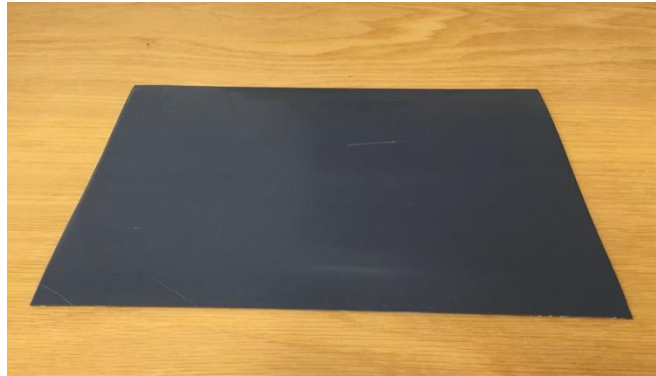
Figure 34: PVC pad used for scenario B. This pad replaced the rear glass of the PV module and was directly inserted for experimentation.
