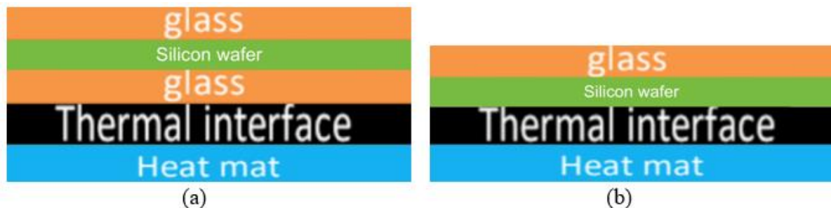
Figure 30: PV/T systems investigated in this report. (a) Scenario A where glass/glass PV module is attached onto the heat mat with a suitable TIM and (b) Scenario B where rear glass of the PV module is replaced by TIM and adhered to the heat mat.
