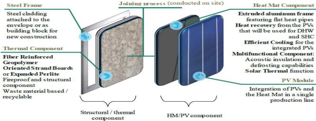
Figure 5: Building block comprising of a PV/T system joined to the structural component for an active building envelope. These two components are produced separately and later assembled together [9].
