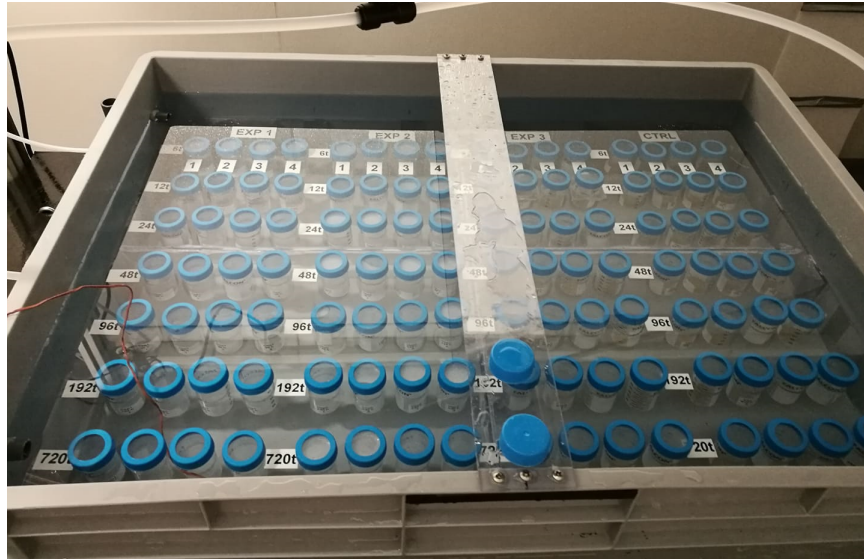
Figure 9: Photo of the recovery rig. After exposure, the samples were placed in the recovery rig for depuration. (Photo: Bjørn Henrik Hansen).
