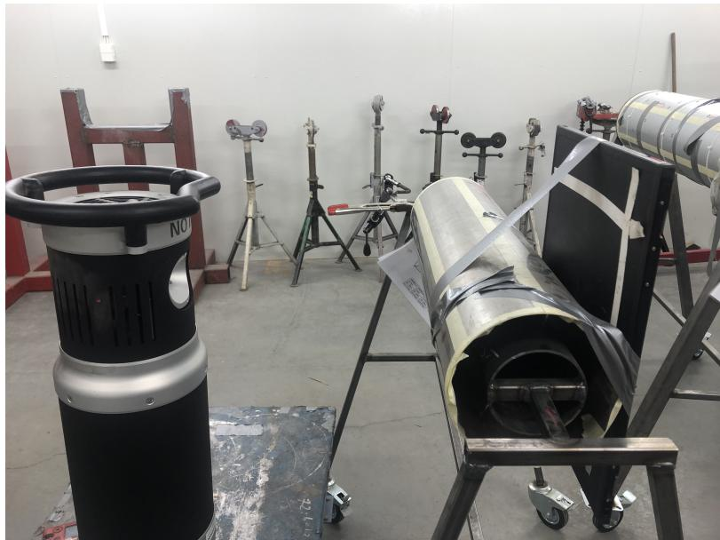
Figure 17: Setup for test object 1 with a 300 kV X-ray tube as radiation source.
