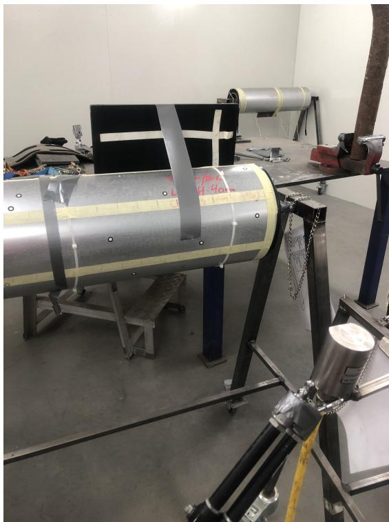
Figure 15: Setup for test object 2 with an Ir-192 isotope as radiation source.
