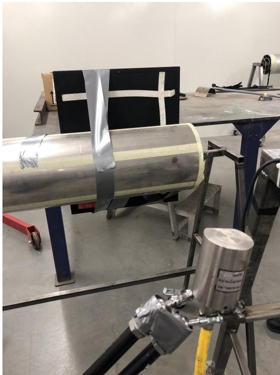
Figure 14: Setup for test object 1 with an Ir-192 isotope as radiation source.
