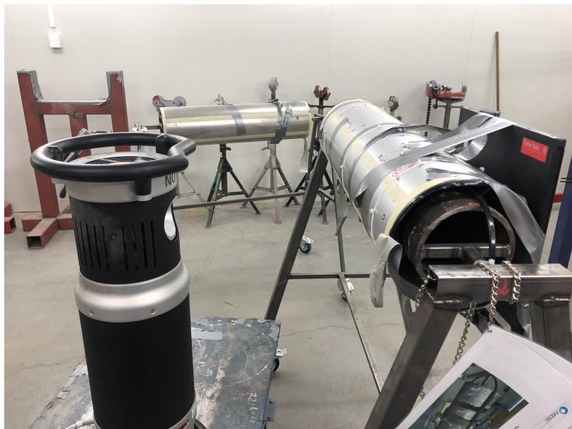
Figure 18: Setup for test object 2 with a 300 kV X-ray tube as source of radiation.
