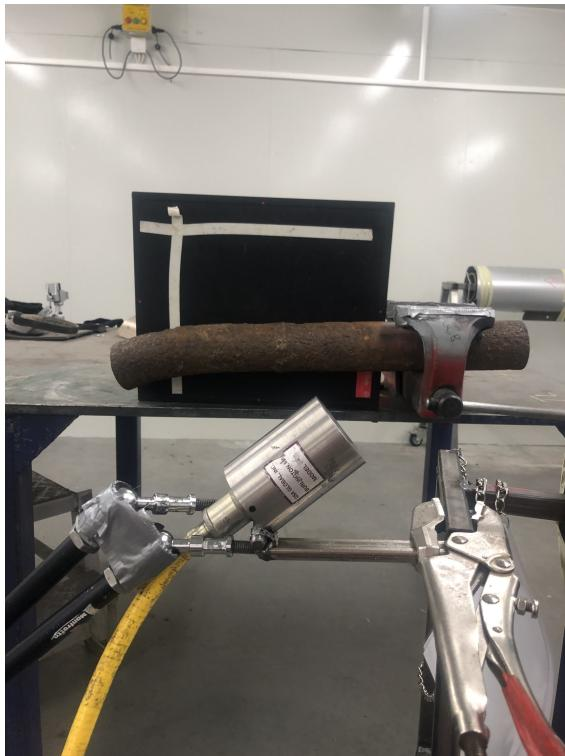
Figure 16: Setup for test object 3 with an Ir-192 isotope as radiation source.
