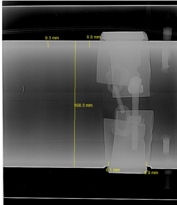
Figure 23: Test object 2 inspected with an Ir-192 isotope.
