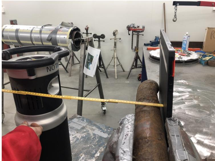
Figure 19: Setup for test object 3 with a 300 kV X-ray tube as radiation source.
