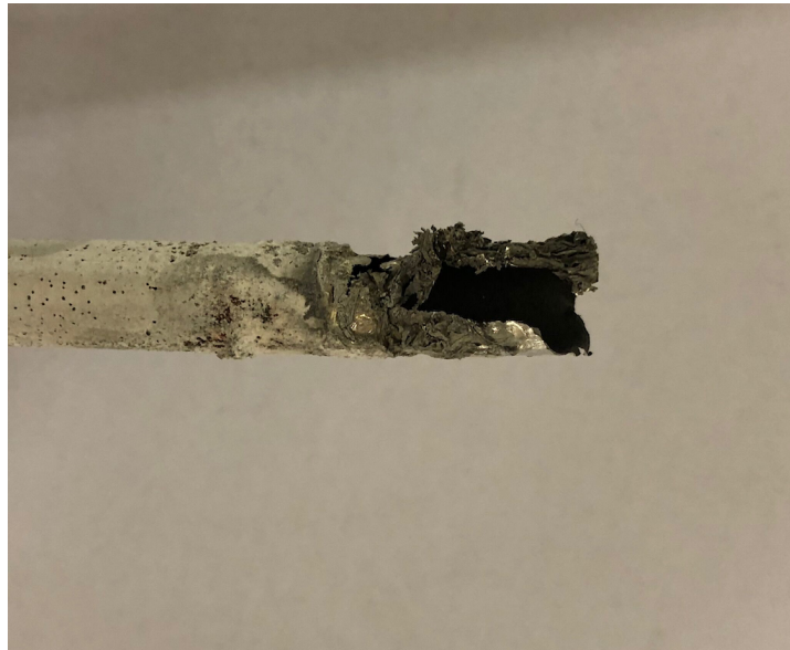
Figure 16: Shows the fracture of the coated stainless steel degassing rod. The rod was subjected to Al-melt for 10-20 minutes at a time.
