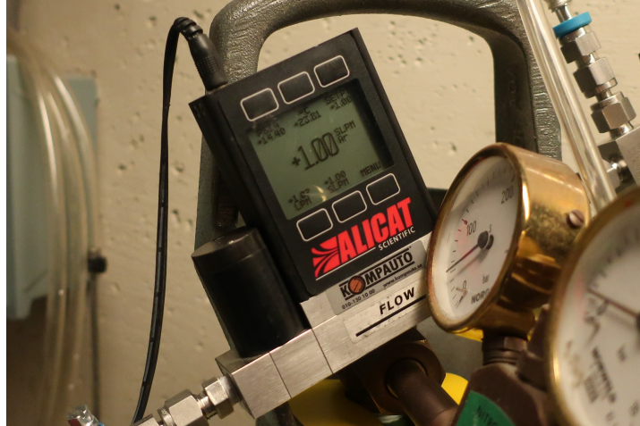
Figure 15: The flow-meter used to control the Ar-gas for purging and degassing.
