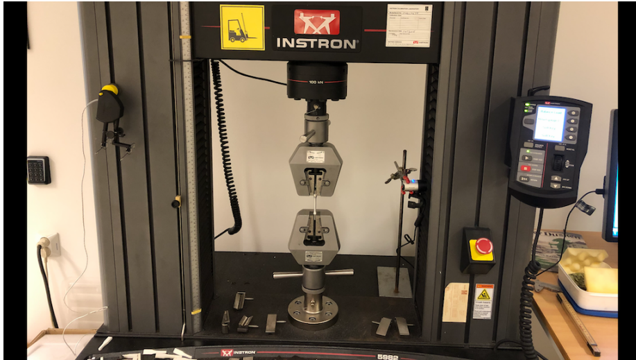
Figure 23: The Instron 5982 machine used to perform tensile tests.
