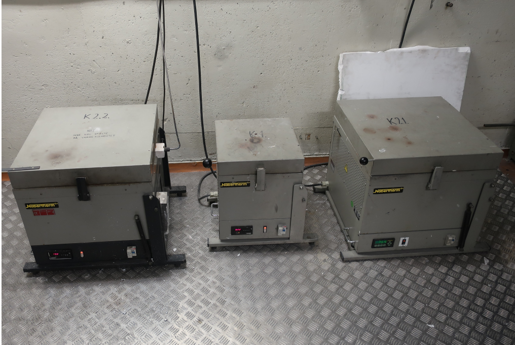
Figure 14: The three Nabertherm furnaces used during the casting trials.
