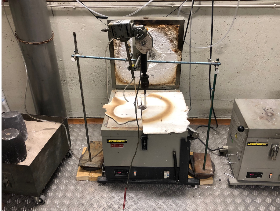
Figure 17: The homemade jig to hold the degassing rod and the engine used for stirring. During stirring and degassing, alumina-fibres were used to cover the open oven, preventing loss of heat.
