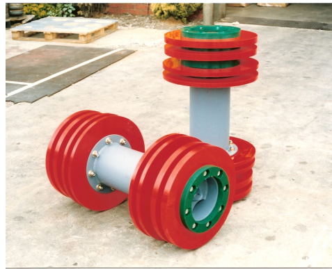
Figure 2.6: Mechanical pigs used to remove deposits along the inside of a pipe line. (HORIZON Industrial Pty Ltd, 2015)
