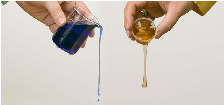
Figure 2.7: Fluids with different viscosity. Fluid one (blue) have a low viscosity, while fluid two (yellow) have a high viscosity. (All Pumps Sales & Service, 2015b)
