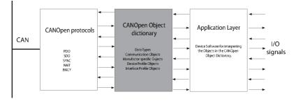
**Figure 2.3:** All parameters are set and read from the CANopen Object Dictionary
