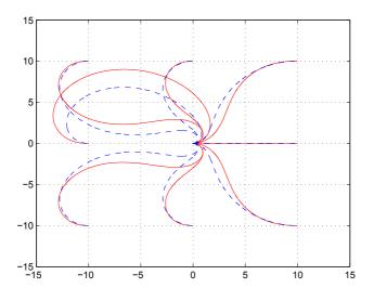
Figure 5.4: How an offset between real and calculated  $\omega$  influences the trajectory of the path. Blu striped lines shows how the vehicle would move without any modelling errors. Red solid lines show how the trajectory of a vehicle where the real world  $\omega$  is 50% lower than the one of the controller.
