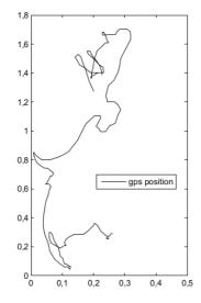
Figure 6.3: Variation of GPS position when vehicle stands still
