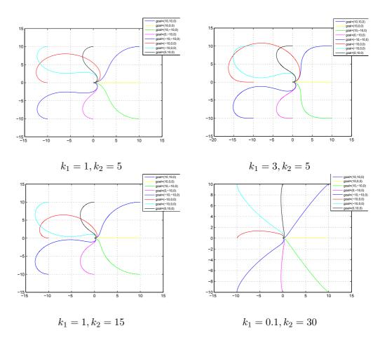
**Figure 5.3:** Trajectories with the proposed control law with different values for  $k_1$  and  $k_2$ . The poses are given as  $(x, y, \theta_P)$  where  $\theta_P$  is the orientation of the vehicle. The initial pose of the vehicle is at (0,0,0) for every trajectory
