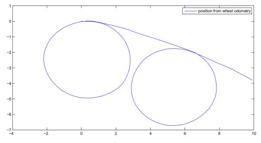
Figure 6.5: Postion from wheel odometry alone
