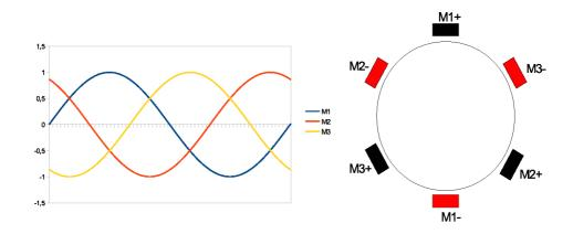
Figure 3.1: Three phase motor
