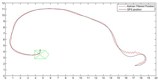
**Figure 6.6:** Kalman filtered position (red), gps position(black) and goal(middle of the green vehicle)
