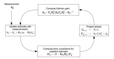
Figure 2.6: Sequential loop in the Kalman filter
