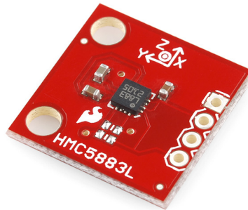
Figure 3.9: HMC5883L is a triple-axis magnetometer. Image provided by sparkfun.com
