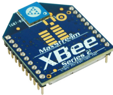
Figure 3.7: The XBee Series 2 is a module using ZigBee as a protocol for wireless communication. Image provided by sparkfun.com
