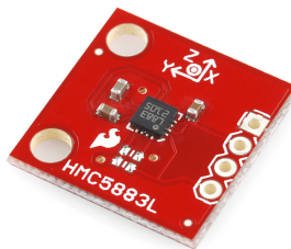
Figure 3.10: HMC5883L is a triple-axis magnetometer. Image provided by sparkfun.com
