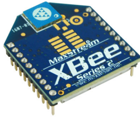
Figure 3.11: The XBee Series 2 is a module using ZigBee as a protocol for the wireless communication. Image provided by sparkfun.com
