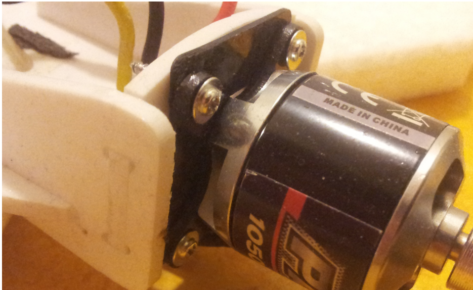
Figure 2.8: Motor mounted through carbon fiber plate
