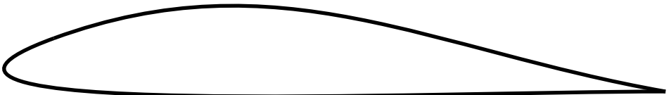
(c) Thick airfoil "high lift"
