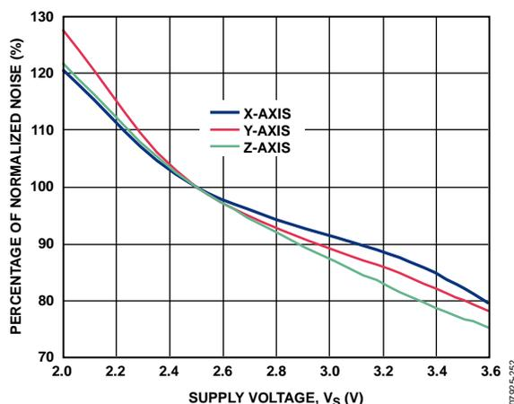
Figure 53. Normalized Noise vs. Supply Voltage,  $V_s$
