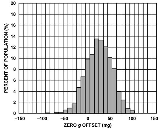
Figure 8. Y-Axis Zero g Offset at 25°C, V<sub>S</sub> = 3.3 V
