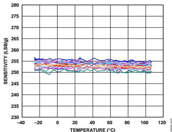
Figure 27. Z-Axis Sensitivity vs. Temperature—
