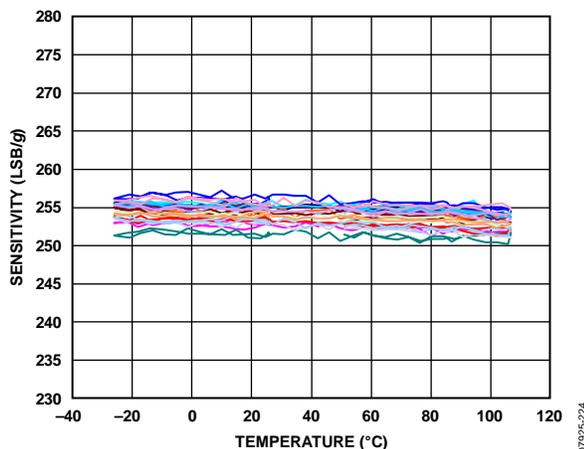
Figure 24. Z-Axis Sensitivity vs. Temperature—
