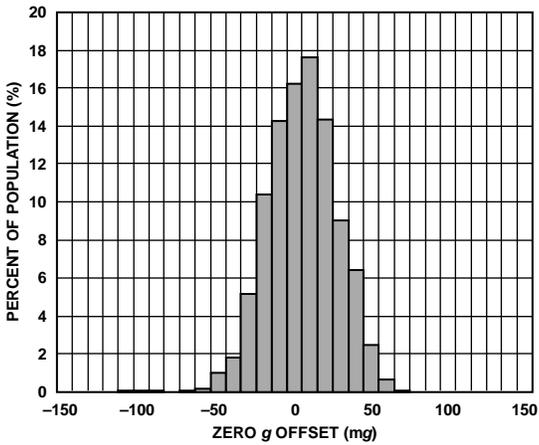
Figure 5. Y-Axis Zero g Offset at 25°C, V<sub>S</sub> = 2.5 V
