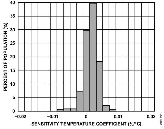
Figure 20. Y-Axis Sensitivity Temperature Coefficient, V<sub>S</sub> = 2.5 V
