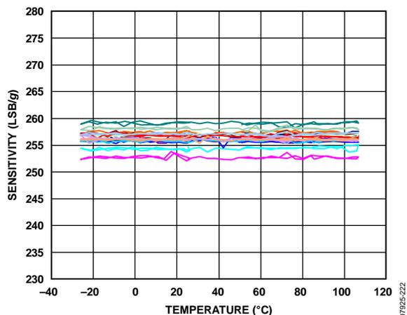
Figure 22. X-Axis Sensitivity vs. Temperature—
