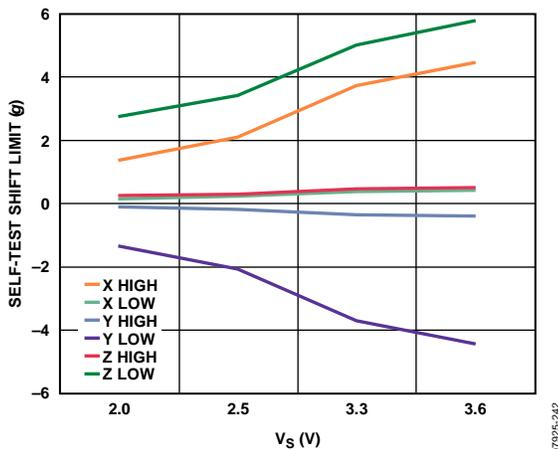
Figure 43. Self-Test Output Change Limits vs. Supply Voltage
