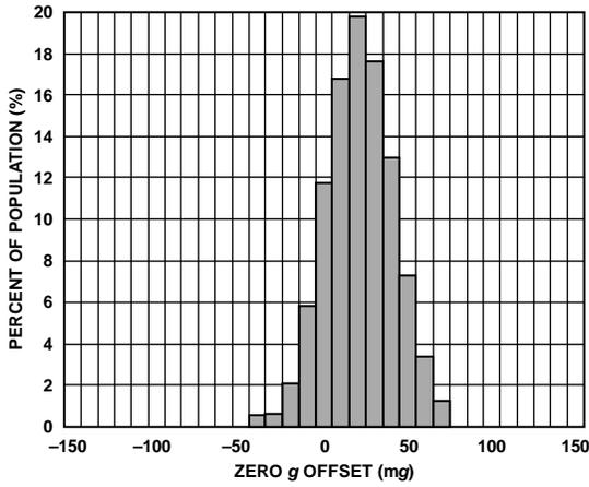
Figure 4. X-Axis Zero g Offset at 25°C, V<sub>S</sub> = 2.5 V
