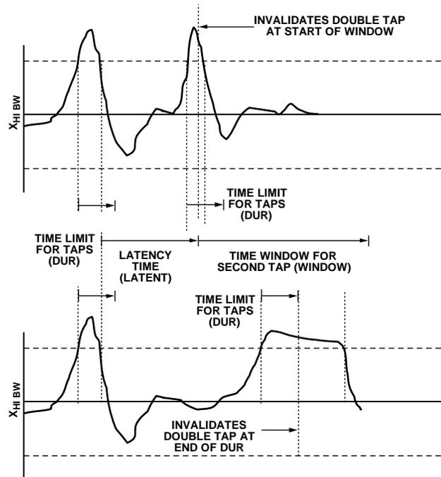
Figure 48. Tap Interrupt Function with Invalid Double Taps
