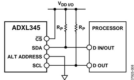
Figure 40. I<sup>2</sup>C Connection Diagram (Address 0x53)
