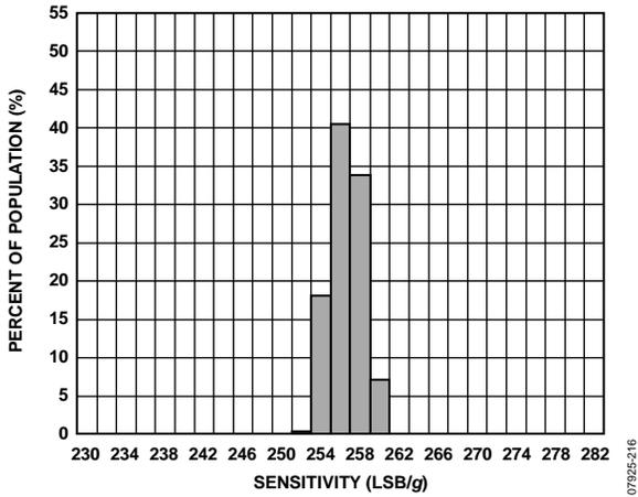
Figure 16. X-Axis Sensitivity at 25°C, V<sub>S</sub> = 2.5 V, Full Resolution
