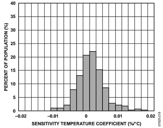
Figure 19. X-Axis Sensitivity Temperature Coefficient, V<sub>S</sub> = 2.5 V
