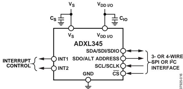
Figure 44. Application Diagram
