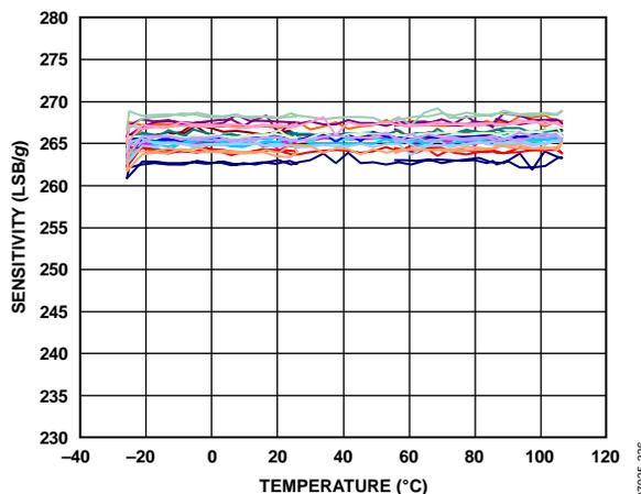
Figure 26. Y-Axis Sensitivity vs. Temperature—
