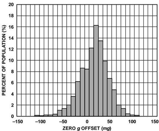
Figure 6. Z-Axis Zero g Offset at 25°C, V<sub>S</sub> = 2.5 V
