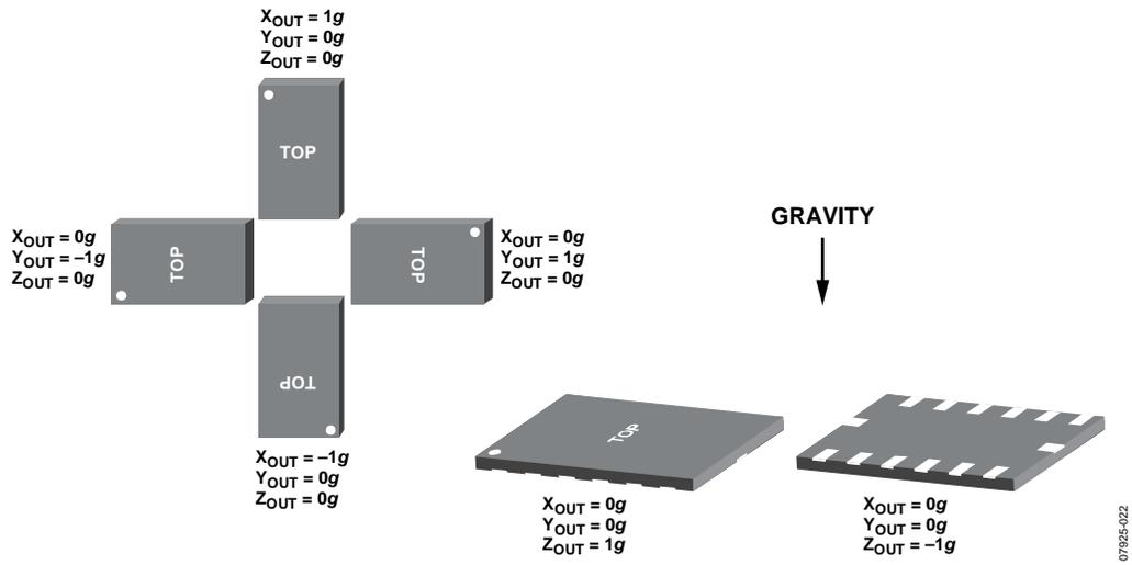
Figure 58. Output Response vs. Orientation to Gravity
