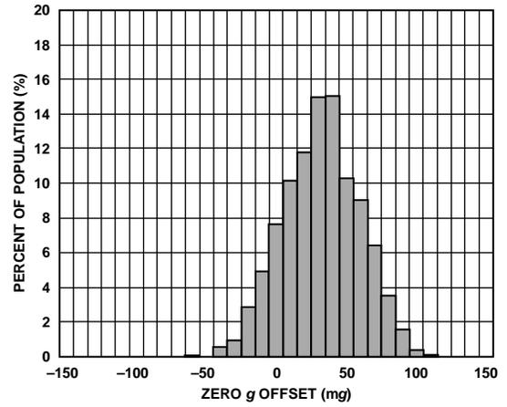
Figure 7. X-Axis Zero g Offset at 25°C, V<sub>S</sub> = 3.3 V
