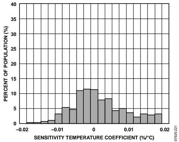
Figure 21. Z-Axis Sensitivity Temperature Coefficient, V<sub>S</sub> = 2.5 V
