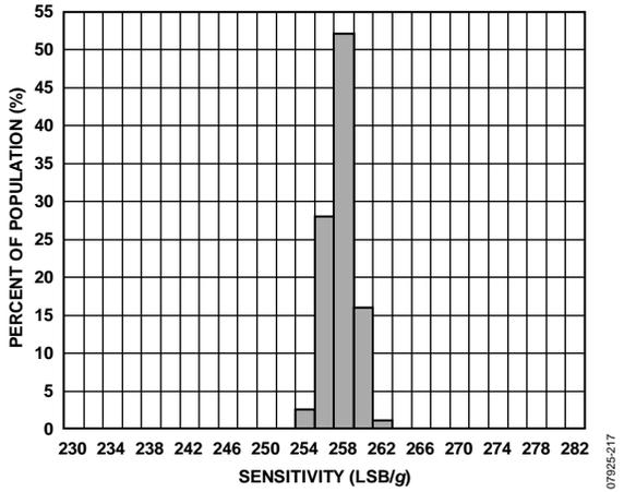
Figure 17. Y-Axis Sensitivity at 25°C, V<sub>S</sub> = 2.5 V, Full Resolution
