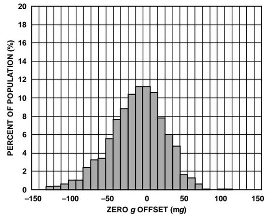
Figure 9. Z-Axis Zero g Offset at 25°C, V<sub>S</sub> = 3.3 V
