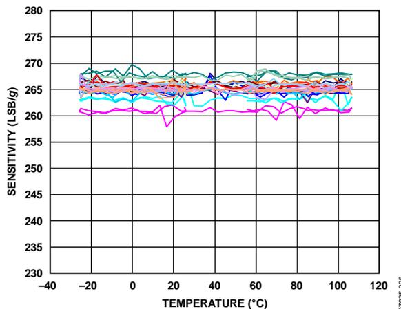
Figure 25. X-Axis Sensitivity vs. Temperature—
