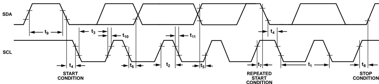
Figure 42. I<sup>2</sup>C Timing Diagram
