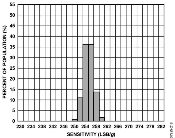
Figure 18. Z-Axis Sensitivity at 25°C, V<sub>S</sub> = 2.5 V, Full Resolution
