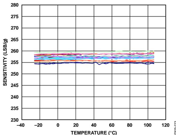
Figure 23. Y-Axis Sensitivity vs. Temperature—
