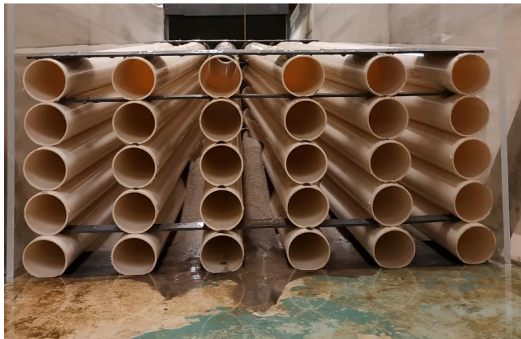
Figure 33 Detail of flow calming structure No. 1 after test 4
