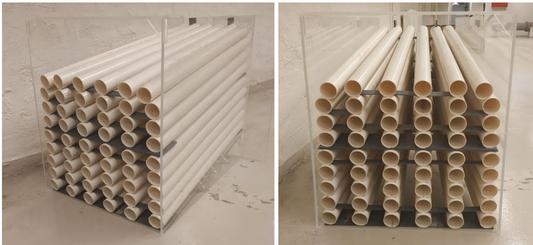
Figure 19 Photo of flow calming structure No. 1
