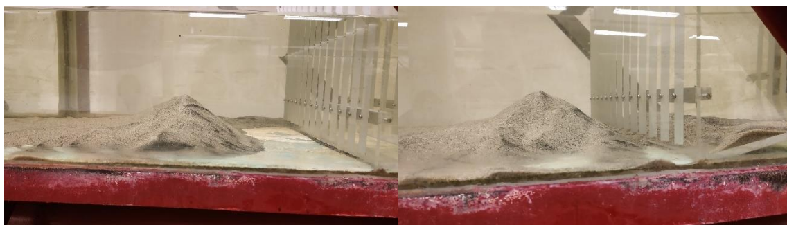
Figure 41 Side view of the sediment's deposition (test 8 on the left side and test 9 on the right side)
