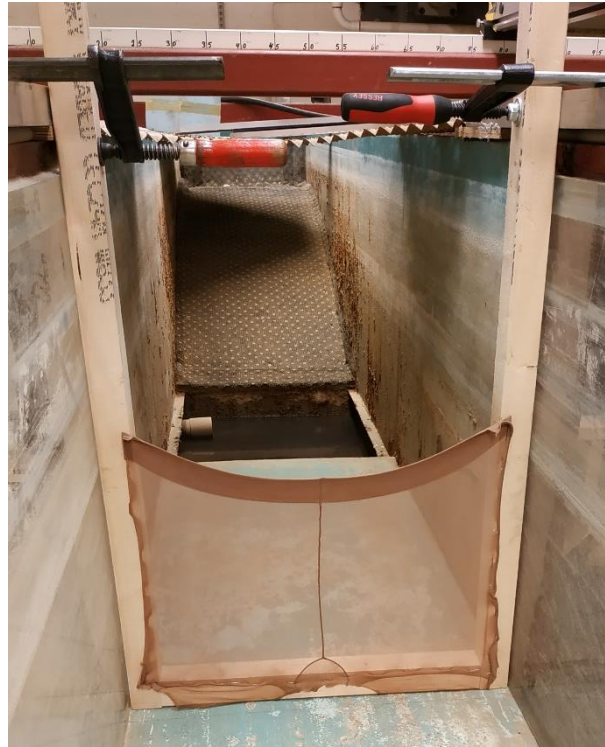
Figure 14 Filter placed most downstream in the flume
