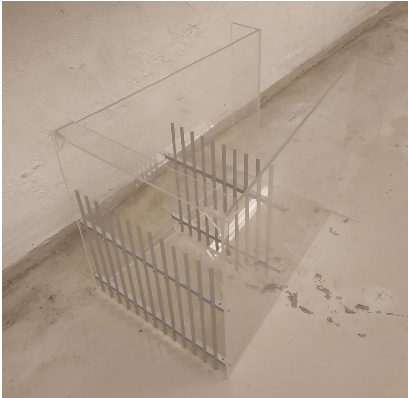
Figure 28 Photo of flow calming structure No. 3, layout 3
