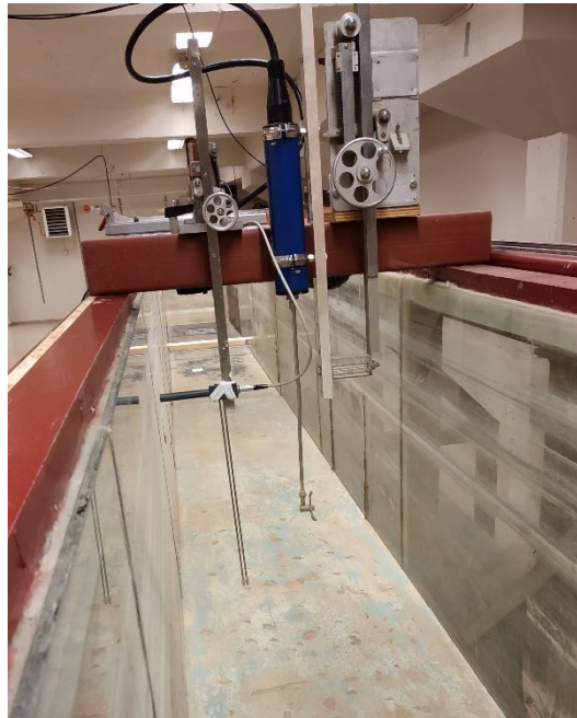
Figure 16 Acoustic Doppler velocimeter installed in the flume
