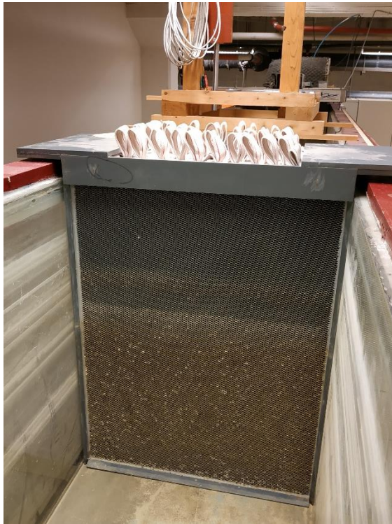
Figure 11 Honeycomb installed most upstream in the flume ensuring stable inflow conditions
