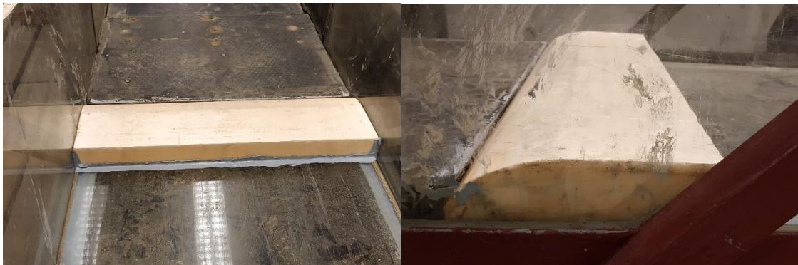
Figure 13 Weir creating the end of the sand trap (view from the upstream on the left side, side view on the right side)
