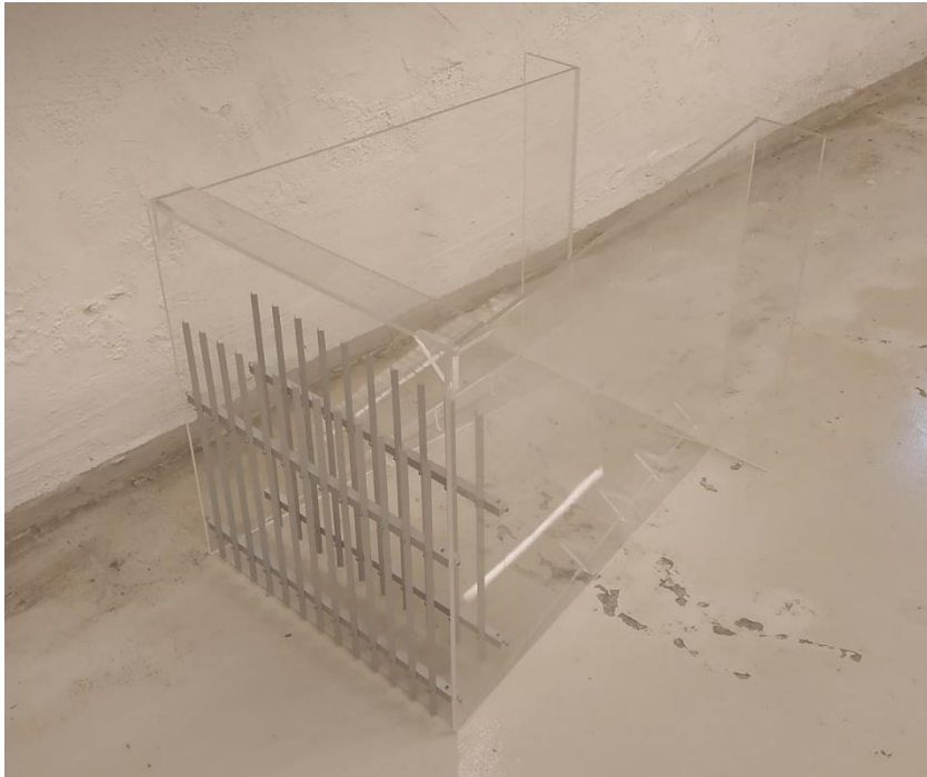
Figure 27 Photo of flow calming structure No. 3, layout 2
