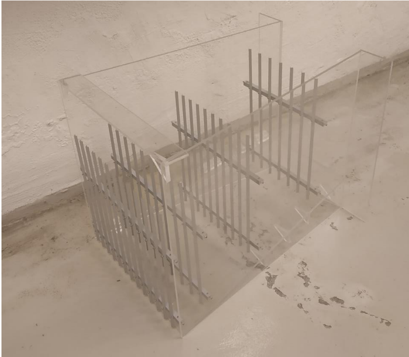
Figure 26 Photo of flow calming structure No. 3, layout 1
