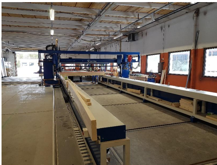
Figur 12: Spikerrobot, Snøhetta element AS
