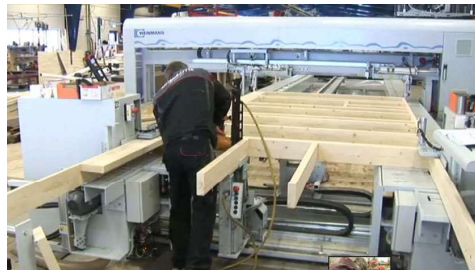
M.0301 – framework construction
