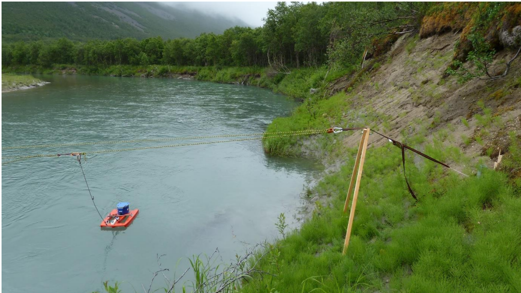
Figure 6: Setup of the moving boat cableway.
