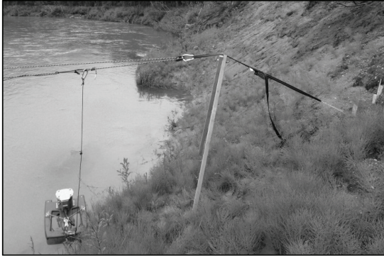
Figure 3: Mounting of mobile cable way for StreamPro ADCP, transect 06, right bank.
