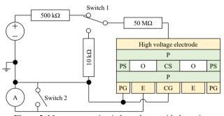
Figure 2. Measurement circuit, here shown with the series connection sample. The sketch is not to scale.
