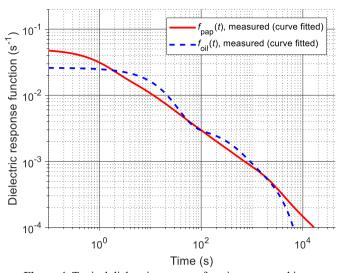
Figure 4. Typical dielectric response function measured in paper and oil, curve fitted to sums of exponential functions (8) and extrapolated backwards. The dielectric response functions shown here were used in the further calculations.
