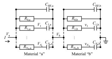
Figure 1. Equivalent circuit of two materials in a series connection. The potentials in the circuit are denoted by V and v.
