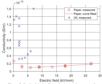
**Figure 3.** Conductivity in oil samples ( $\sigma_{oil}$ ) and paper samples ( $\sigma_{pap}$ ). Curve fitted  $\sigma_{pap} = \sigma_0 \exp(\eta E_{pap})$  with  $\sigma_0 = 8.61 \times 10^{-15}$  S/m and  $\eta = 0.0280$  mm/kV from  $E_{pap} = 5$  kV/mm and above. Average  $\sigma_{oil}$ : 0.841 × 10<sup>-13</sup> S/m. Data for  $\sigma_{oil}$  are previously published in [12].
