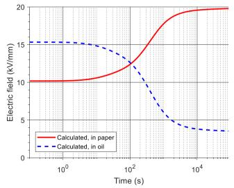
Figure 5. Calculated electric field in paper and oil in the series connection sample.
