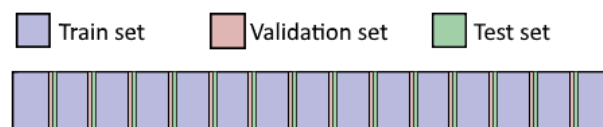
Figure 8.12: Deterministic split of a dataset into a train, validation and test set.
