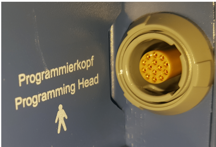
Figure 4.9: 14-pin port for Redel P series adapter to connect the programming head
