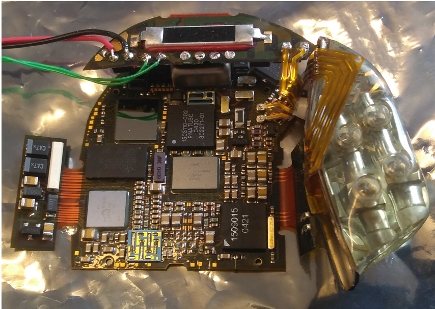
Figure 5.1: Pacemaker with outer components desoldered giving access to the underlying chips.
