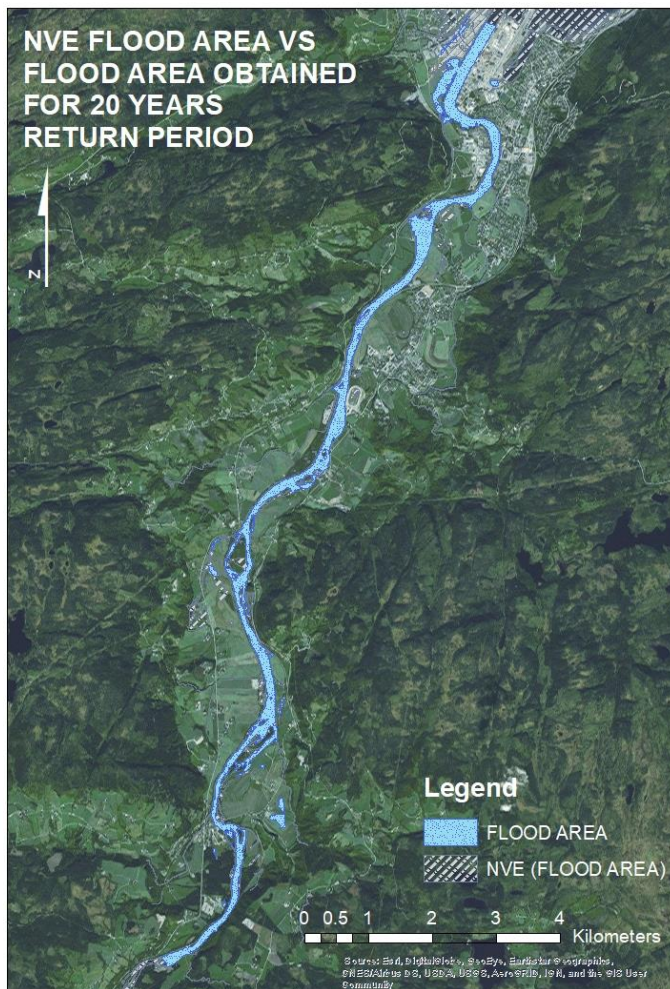
Figure 24: Comparison between the flood area obtained in this thesis and the flood area of NVE for 20 years return period
